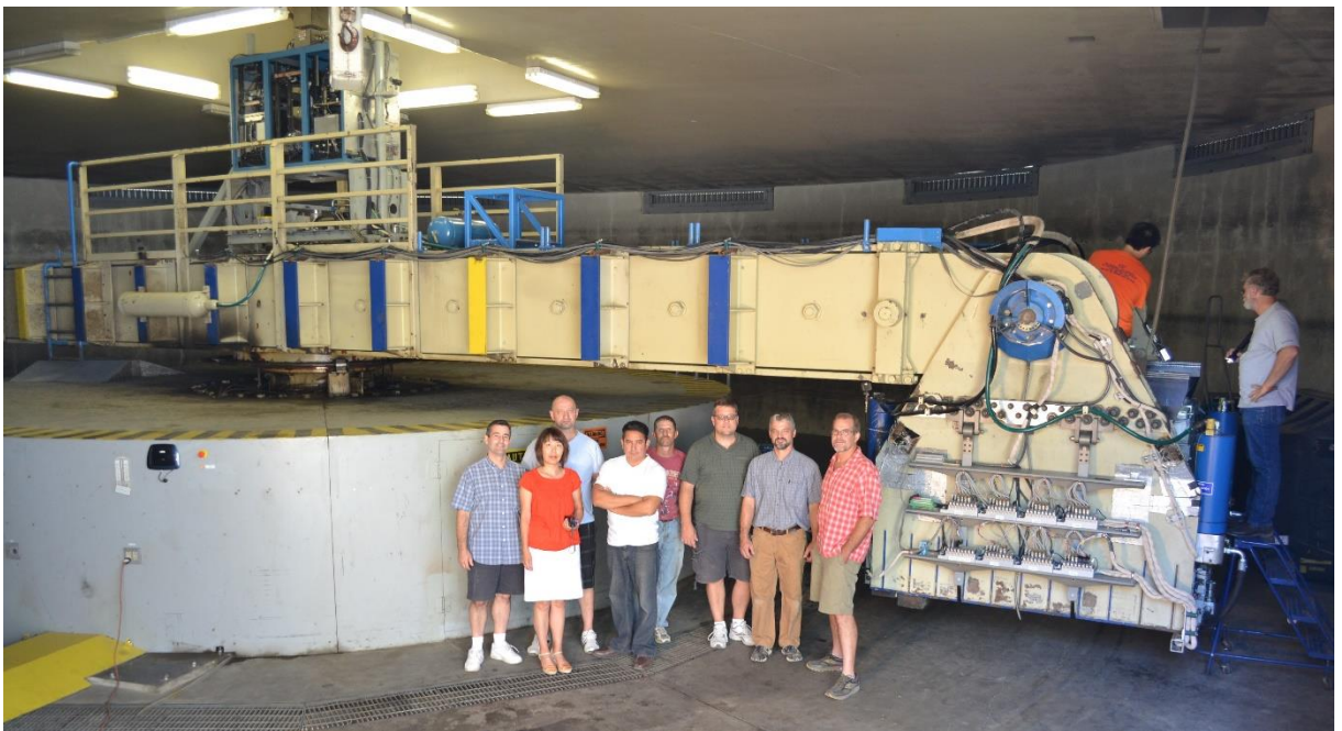
Figure 35 Centrifuge med 9m radius (oppgradert), Center for Geotechnical Modeling, UC Davis, California
