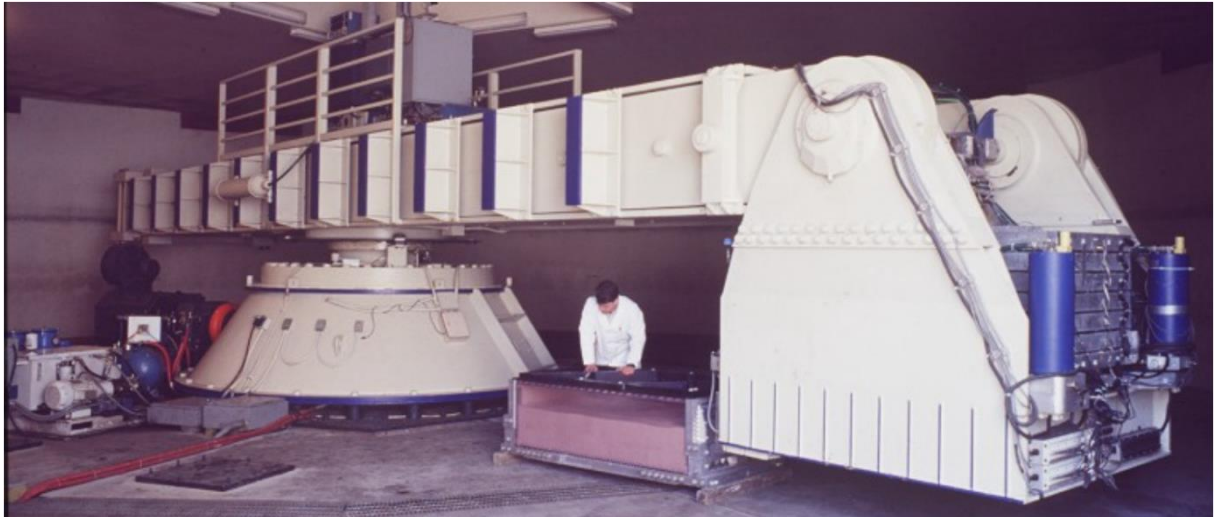
Figure 34 Geotechnical centrifuge at the University of California, Davis, 9m-radius (30 ft)
