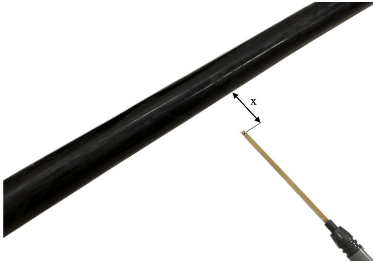
Figure 3.4: The positioning of the Gaussmeter during the validation testing. The probe is positioned perpendicular and centered to the cable with the possibility to adjust the distance.
