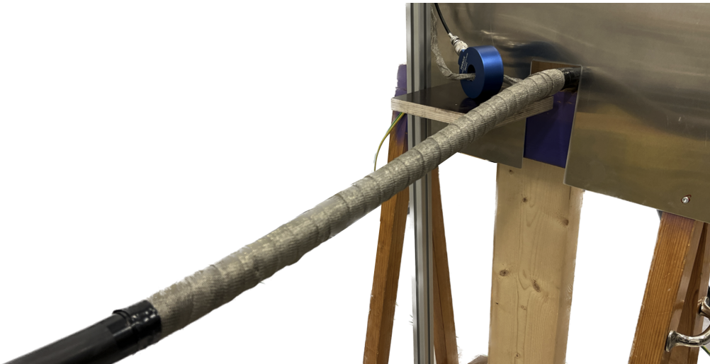
Figure 3.2: Photo of the test object during the 50 Hz experiment. The test object consists of the inductive partial discharge through the use of a HFCT.
