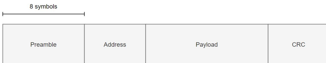
Figure 11: A BLE packet consisting of an 8 bit preamble, an address, a payload and CRC.
