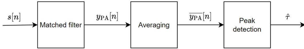
Figure 35: A block diagram of the time domain preamble detector. It is based around a matched filter which is matched to the preamble, and computes the estimate \hat{\tau} using averaging and peak detection.
