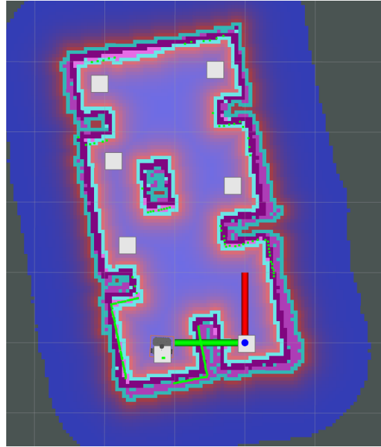
Figure 5.11: Occupancy grid map with waypoints illustrated as white squares. Upper left and lower right waypoints are chargers, with the rest being objects of interest
