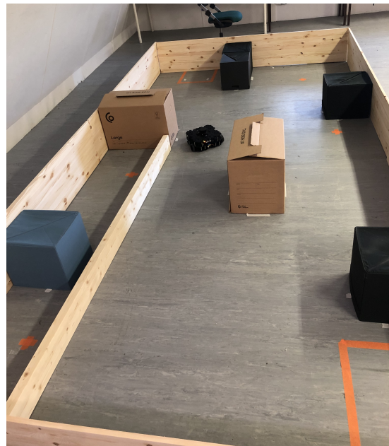
Figure 5.12: Test area with waypoint 3 and 5 blocked by wooden board. The narrow passage between the board and the cardboard box made path planning extra challenging.
