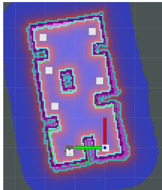
Figure 4.6: Screenshot from Rviz showing the occupancy grid map for the test area with the global costmap (colored overlay) and waypoints (white squares).
