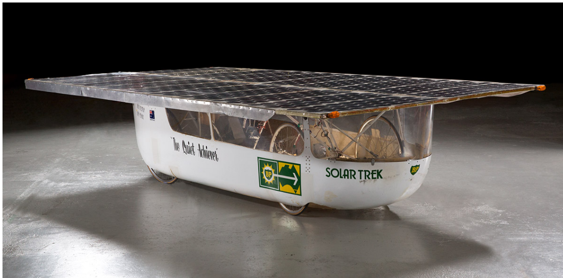
Figure 1: The Quiet Achiever. Worlds first practical SC powered entirely by PV-cells.
