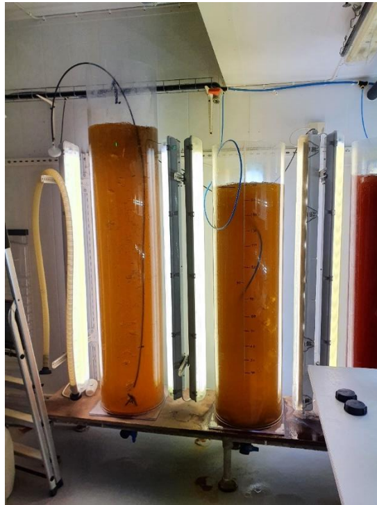
Figure 6 – Bioreactors used to produce microalgae Tisochrysis. lutea . The culture was continuously supplied with carbon dioxide.
