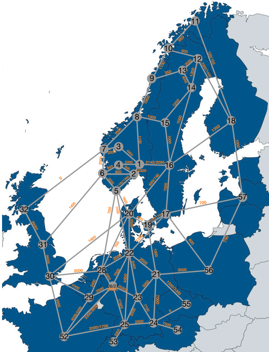
Figure 6: Transmission capacity in MW for the lines connecting the onshore areas
