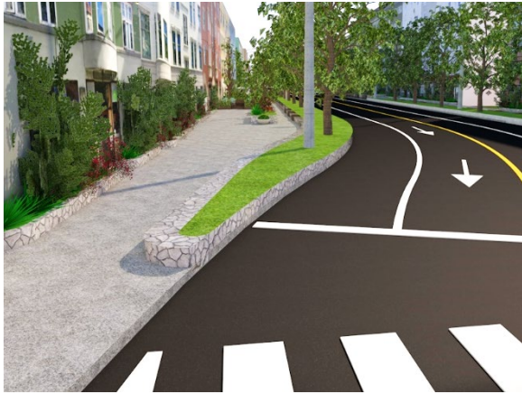
Figure 9-16: Render from model showing an example of an elevated green divider. (Made by: Susanna Hsu Hals)
