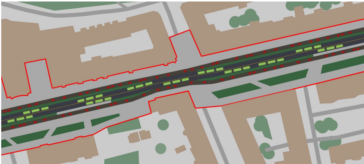
Figure 8-4: Public transport lanes in the middle of the road. (Made by: Susanna Hsu Hals)
