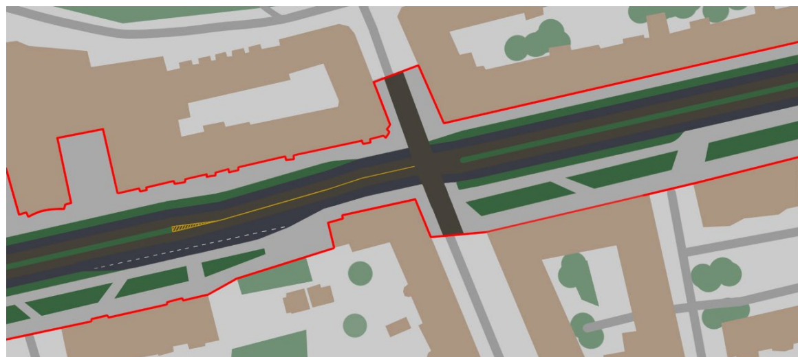
Figure 8-3: Green dividers and green areas on the sidewalk. (Made by: Susanna Hsu Hals)
