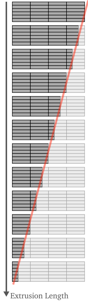
Figure 41: The figure illustrates how the proper allocation of variables for the billet cells throughout the NLP horizon contributes to reducing the necessary number of NLP variables. The dark cells indicate ‘active’ cells, and light cells indicate ‘dead’ cells. The red line illustrates how the number of active cells are nearly half the total number of cells.
