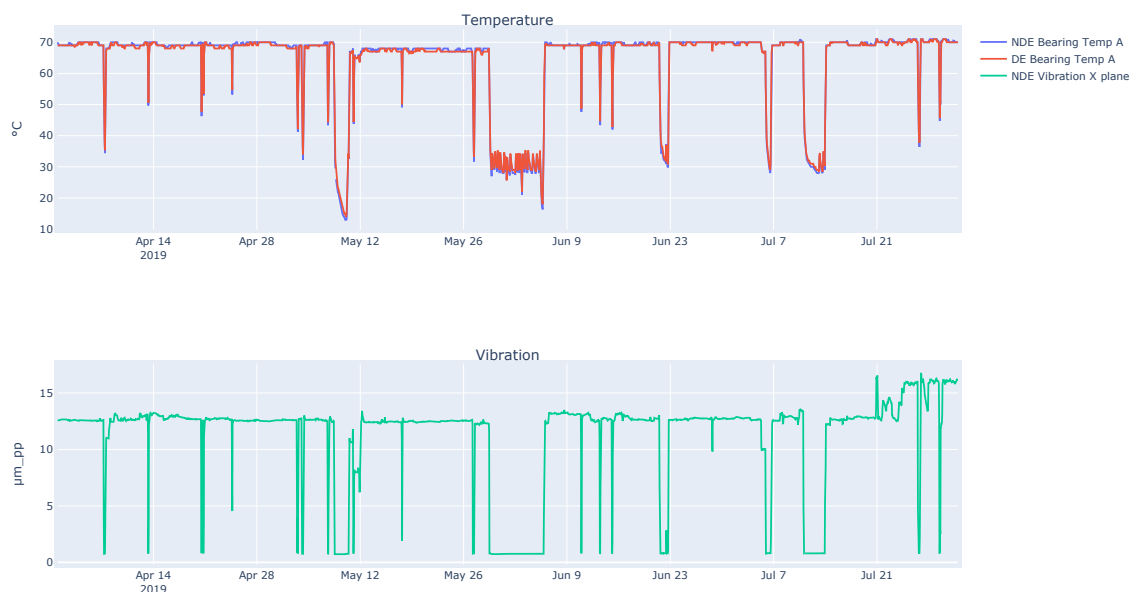
Figure 26: The bearing temperatures and vibration.
