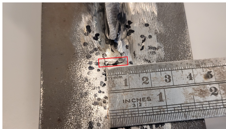
Figure 5.6: Initiation of crack on the opposite weld toe
