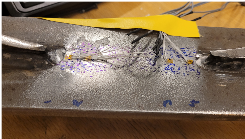
Figure 4.3: Strain gauges mounted on the test specimen.
