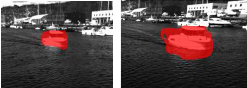
Figure 5.1: The detection of Havfruen in a sequence of images. The left image shows an image early in the sequence while the image to the right shows how Havfruen has moved closer to milliAmpere 1 later in the sequence. The masks are covering Havfruen well, with some deviations. The camera movements are more or less uniform during the sequence.
