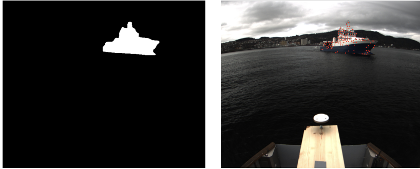
Figure 5.6: A mask of Gunnerus and key points in the mask from the detection in the right image in Figure 5.5. The mask of Gunnerus is chosen manually, as there is more than one mask in the image. The mask fits Gunnerus well, and all points are located on the boat. The points are found with the OpenCV function goodFeaturesToTrack .
