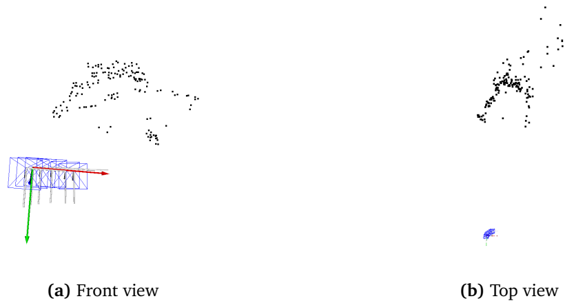
Figure 6.23: Effects of the short baseline on point cloud and consequent pose estimation, due to limited images used for reconstruction. In the front view (left), the ship appears well-structured, falsely indicating a successful reconstruction. However, the top view (right) unveils the true state of the 3D model, exhibiting a skewed orientation not discernible from the front. This demonstrates the intrinsic inaccuracies of the 3D model, manifesting the challenges posed by the short baseline and a limited number of images in capturing the genuine 3D structure of the ship.
