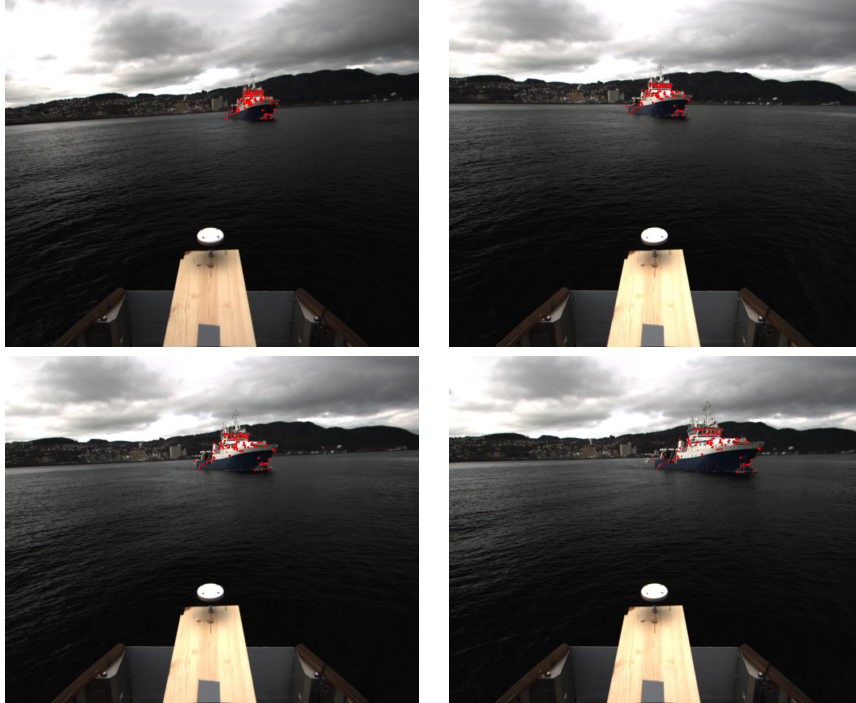
Figure 6.1: A sequence of images where LK is used to track points. The initial points are selected from a mask in the bottom right image. In the sequence, images two seconds apart have been chosen to be able to see the difference between the images.
