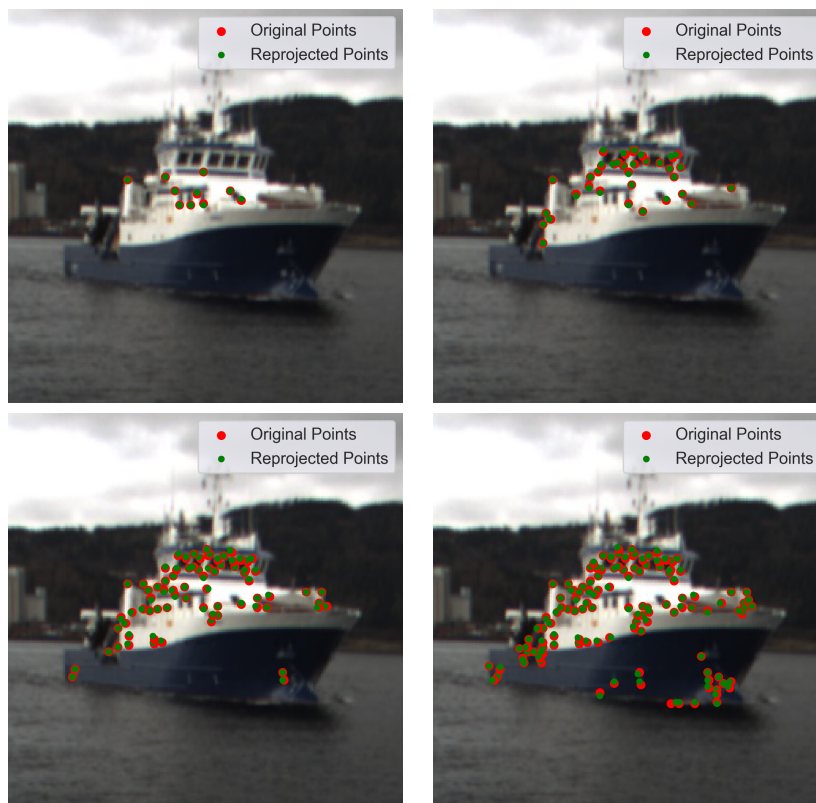
Figure 6.15: Illustration of projected points on an image of Gunnerus in Environment 1, for the varying maximum number of points used in the reconstruction. From top-left to bottom-right, the number of points used are 10, 50, 100, and 200, respectively. It is observed that the reprojection gets slightly worse when more points are used for reconstruction.
