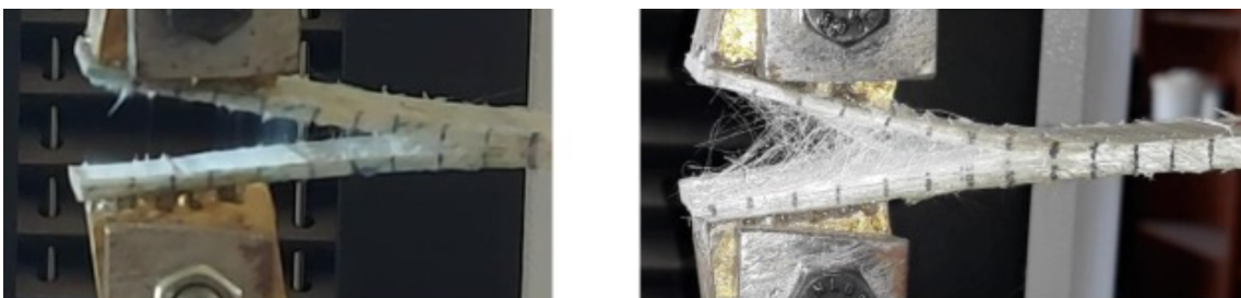
Figure 8: Left: Delamination without bridging. Right: Delamination with fiber bridging. [11]
