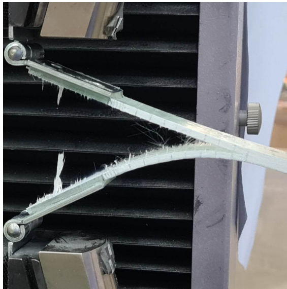
Figure 42: The underside of the specimen bends much more than the top. This is due to the different layups on each side of the crack.
