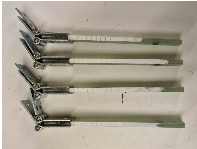
Figure 22: Glass-fiber/Epoxy specimens ready to be tested with mounted hinges, and coated and marked on the side.
