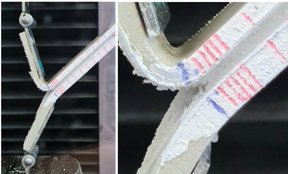
Figure 41: Behavior of the improved slit specimen, and the small delamination acquired.
