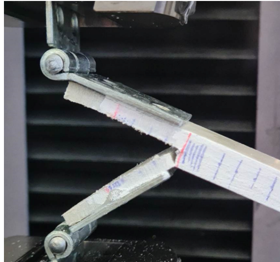
Figure 39: Failure of the initial polypropylene specimens.
