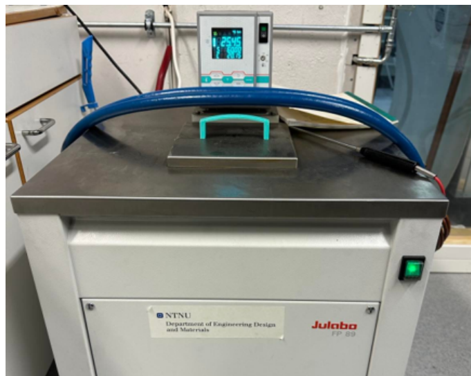
Figure 49: The machine used to age the specimens.
