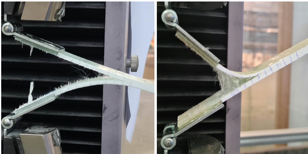
Figure 46: The difference in bending, where the top side of the unaged specimen is bent and the bottom of the aged specimen is bent. From the left: Unaged specimen, Aged specimen.
