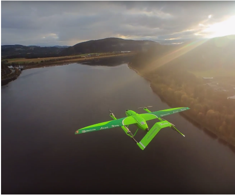
(a) In fixed-wing flight, efficiency is attained through the utilization of forward airspeed and wings to generate lift.
