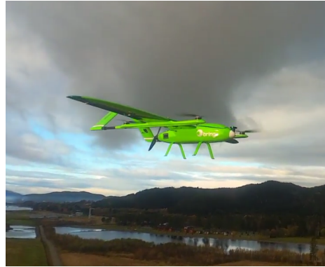
(b) In multirotor flight, the aircraft possesses the capability to achieve vertical takeoff and landing, as well as hover in a stationary position.
