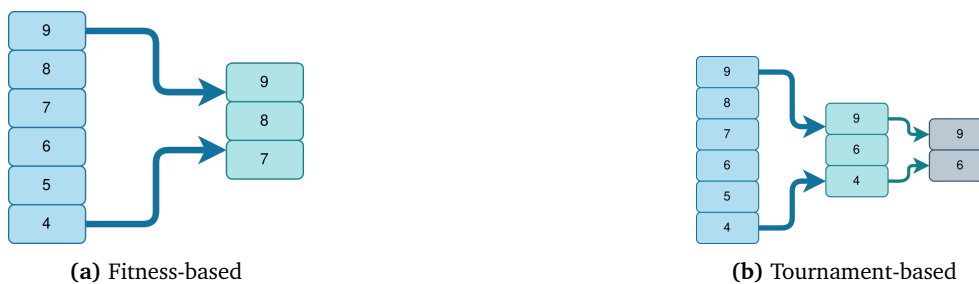
Figure 2.9: Representation of the selection operator on a set of 6 individuals with a given fitness score. In (a) only the individuals with the best fitness can reproduce, while in (b) random individuals are first picked, and then sorted.
