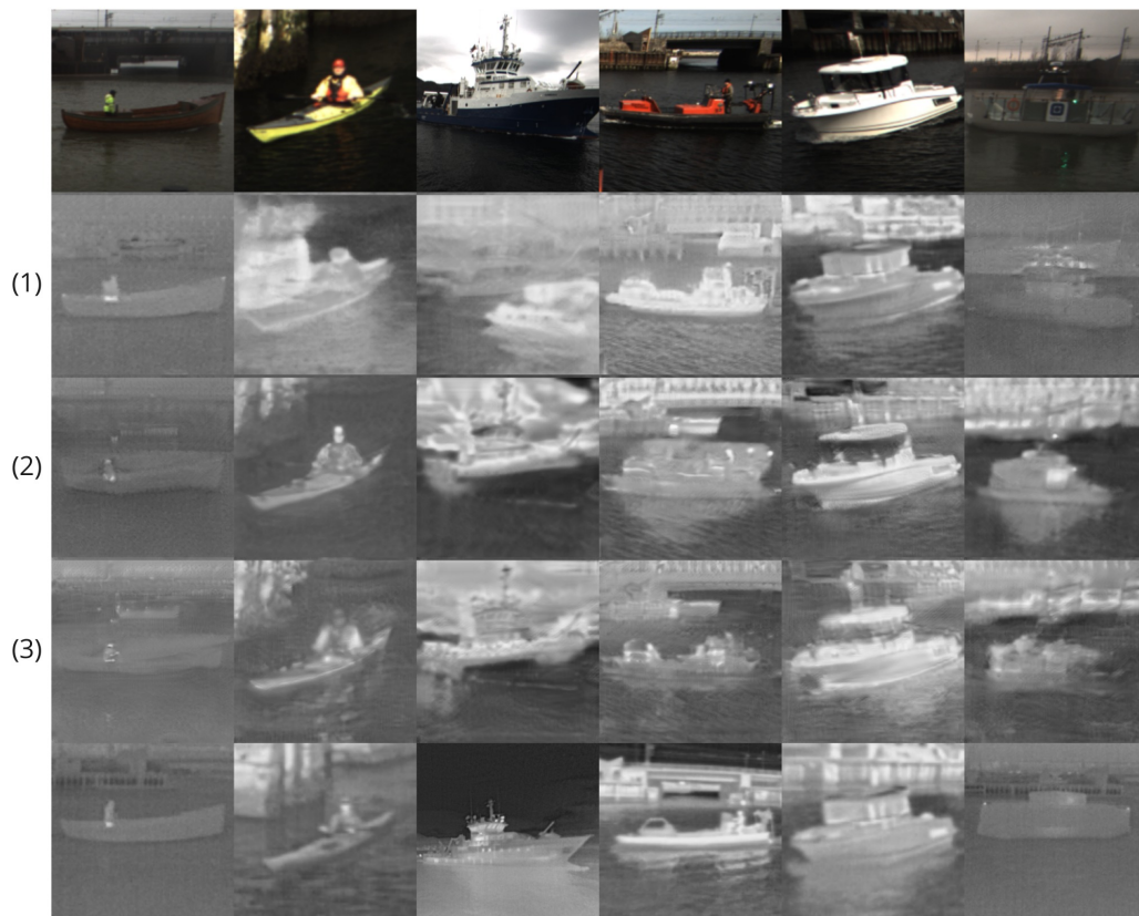
Figure 5.10: The first (source) and last (reference) row presents six hand-picked RGB images from the validation set used to evaluate the translation quality for each object in their respective domain. The intermediate rows show baseline model generations trained on (1) 256x256 images, (2) 196x196 images, and (3) 128x128 images sampled from the final checkpoints.
