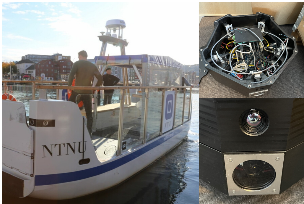
Figure 1.1: Overview of milliAmpere and its camera components. Left-image shows the ferry itself. Top-right shows the electronic box capsuling the various EO and IR cameras. Bottom-right shows the dual-camera setup of a single angle with the infrared lens at the top and electro-optical at the bottom. Left-image is sourced with approval from Universitetsavisa by photographer Oda Eriksen Haugland.
