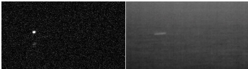
Figure 1.2: Illustration showcasing the visibility of the boat taken with an electro-optical (left-side) and infrared (right-side) camera in pitch-dark environments. Image is sourced from [16] with permission.
