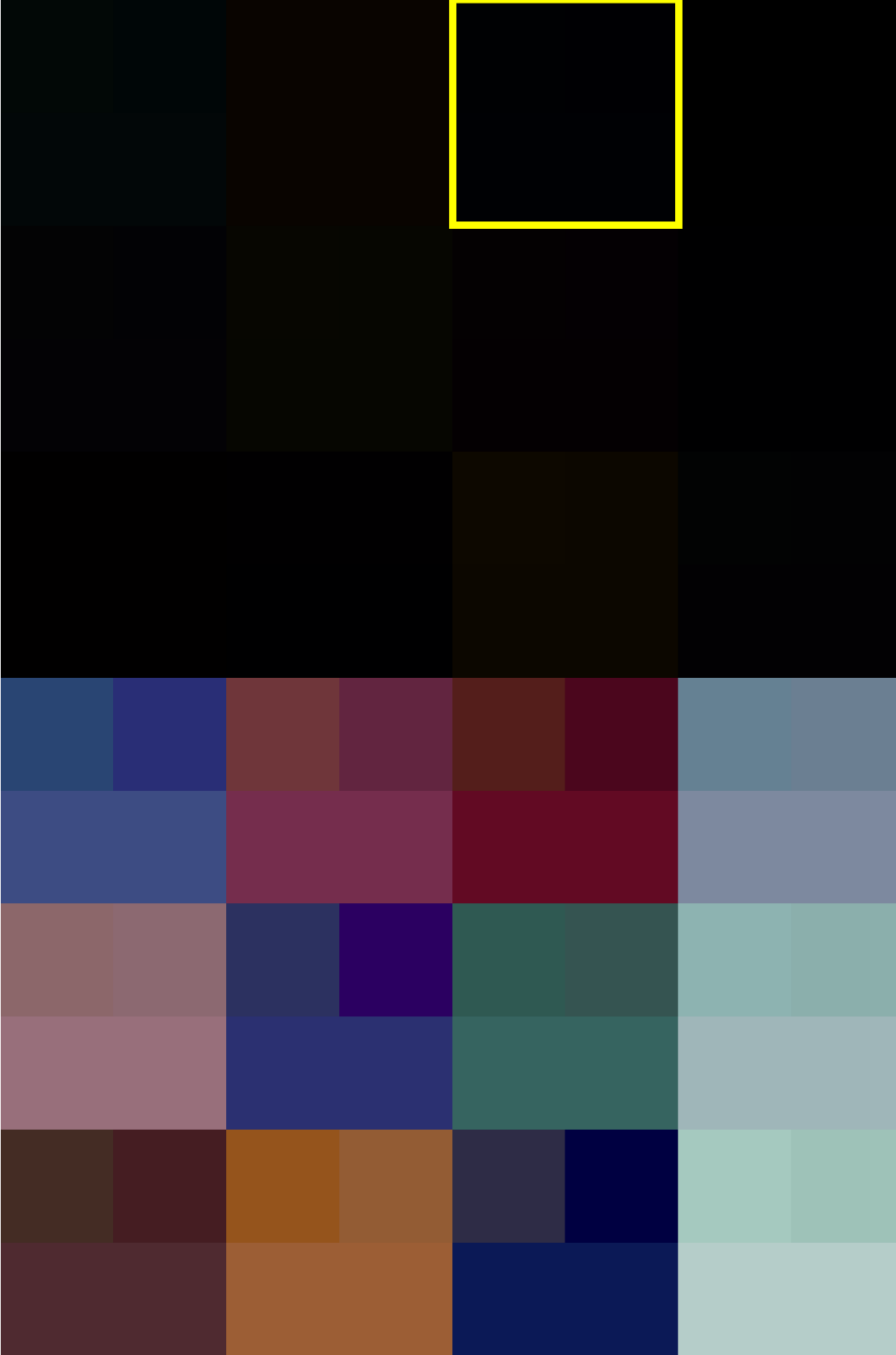
Figure 8.13: Test data reproduction from groundtruth data and predictions from HDR-Dual-RGB and HDR-Dual-RGB-PSO imaging. Each patch consists of four blocks in the form \begin{pmatrix} GT & DRP \\ GT & DRP \end{pmatrix} , where GT is for ground truth, DRP for HDR-Dual-RGB-PSO, and DR for HDR-Dual-RGB block. The tristimulus data is produced by converting to sRGB colourspace, scaling and quantizing the data to 8-bits. The yellow boundary represents out-of-gamut-colour for sRGB colour space
