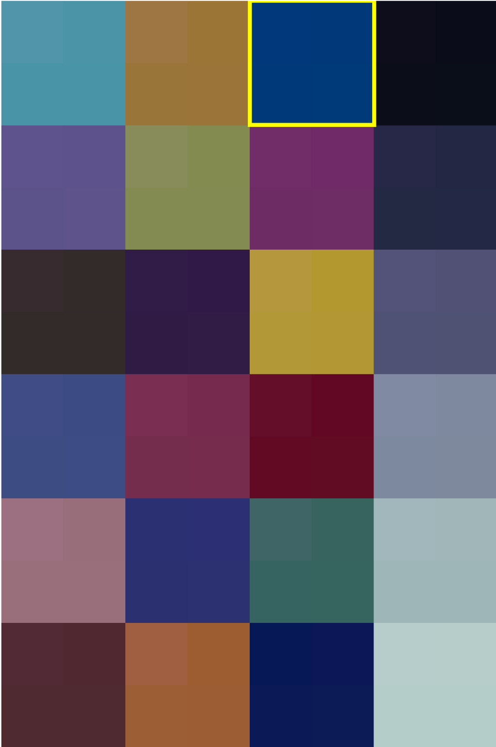
Figure 6.11: Test data reproduction from groundtruth data and predictions from dual-RGB and three-channels imaging. Each patch consists of four blocks in the form (\begin{smallmatrix} GT & TC \\ GT & DR \end{smallmatrix}) , where GT is for ground truth, TC for three-channel and DR for dual-RGB block. The tristimulus data is produced by converting to sRGB colourspace, scaling and quantizing the data to 8-bits.
