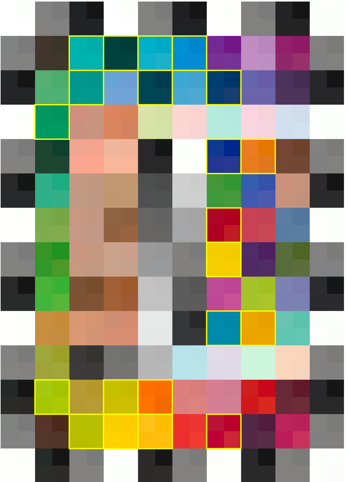
Figure 9.10: Train data reproduction from ground-truth data and predictions from dual-RGB, dual-RGB-PSO and dual-RGB-PSO (light sources optimized for films) imaging. Each patch consists of four blocks in the form (\begin{smallmatrix} GT & DRPT \\ DRP & DR \end{smallmatrix}) , where GT is for ground truth, DRPT for dual-RGB-PSO (light sources optimized for films), DR for dual-RGB, and DRP for dual-RGB-PSO block. The tristimulus data is produced by converting to sRGB colourspace, scaling and quantizing the data to 8-bits. Patches with yellow boundaries are out-of-gamut chromaticities for sRGB colour space limiting the actual demonstration.
