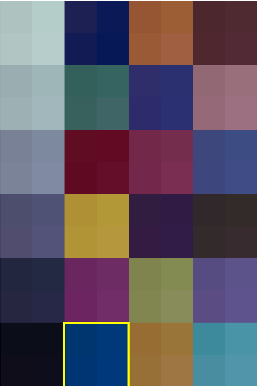
Figure 7.10: Test data reproduction from ground-truth data and predictions from dual-RGB and three-channels imaging. Each patch consists of four blocks in the form (GT TC) , where GT is for ground truth, TC for three-channel, and DR for dual-RGB block. The tristimulus data is produced by converting to sRGB colour-space, scaling and quantizing the data to 8-bits. Patches with yellow boundaries are out-of-gamut chromaticities for sRGB colour space limiting the actual demonstration. The patches with red boundaries are the outliers which are detected in the real and simulated digital numbers correlation plot.
