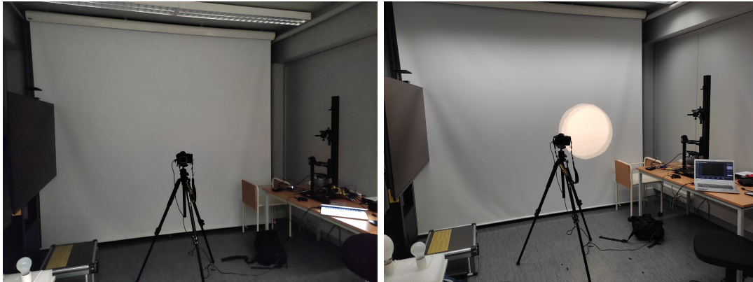
(a) Camera pointing at the white projector screen (b) Projector screen illuminated with three halogen lamps
