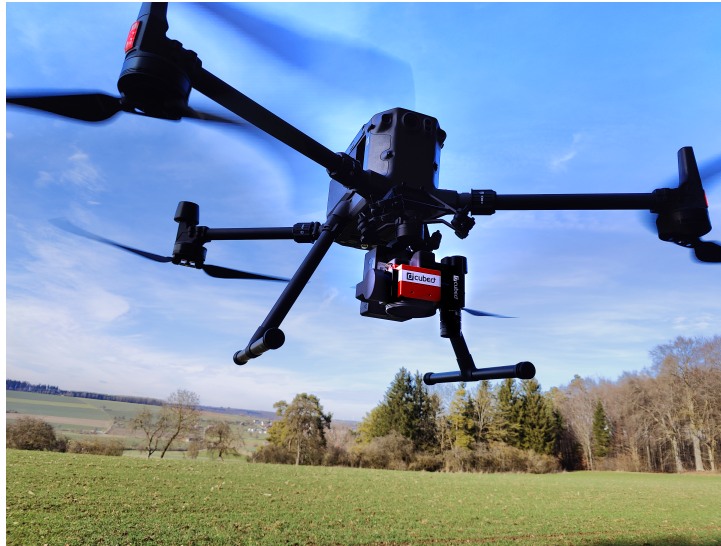
Figure 3.12: Cubert Ultris X20P, including an additional panchromatic sensor, mounted on a UAV mid-flight.
