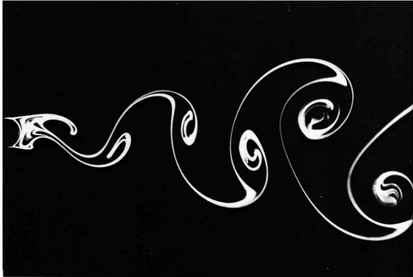
Figure 3: Kármán vortex street in the wake of a circular cylinder at Re = 140 (Van Dyke et al., 1983)
