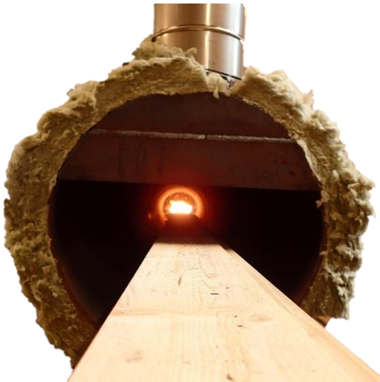
Fig. 2. A wood panel through the thermally insulated steel pipe gets charred at the end.
