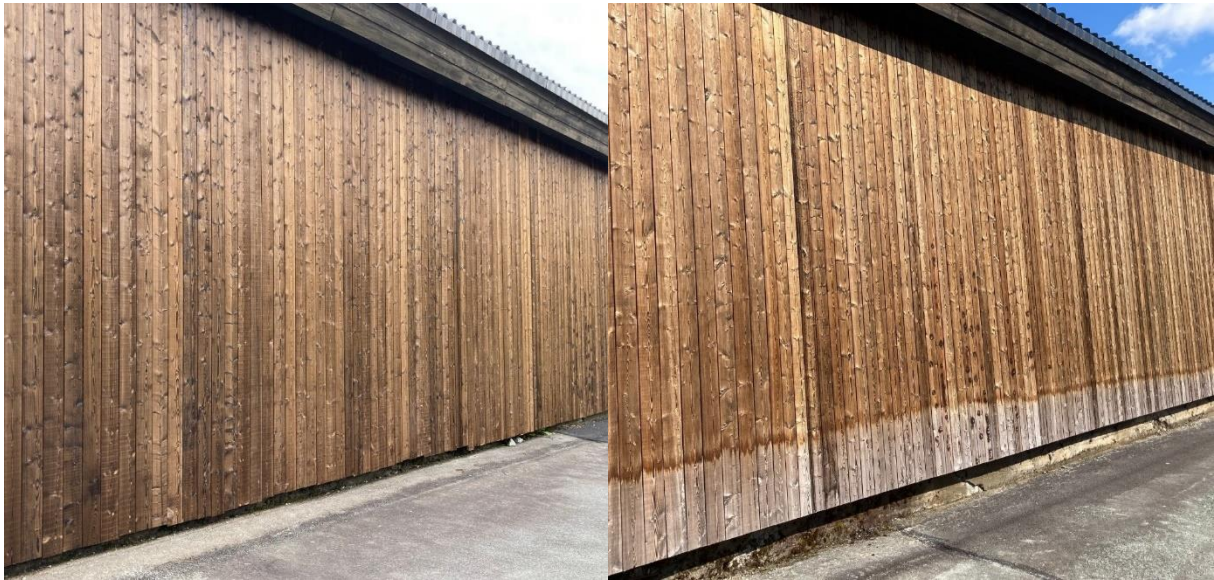
Fig. B1. Left: The test wall when installing 8th of June 2022. The edges were cut right after the picture was taken. Right: Picture of the test wall taken 28th of April 2023 showing a color change along the edge.
