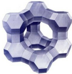
Figure 5: Figure showing the structure of molecular sieve type X . Figure from [Rathish et al. 2013]
