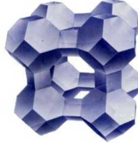
Figure 4: Figure showing the structure of molecular sieve type A. Figure from [Rathish et al. 2013]
