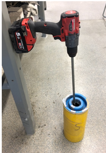
Figure 2.8: The equipment which is used for mixing the matrix for the FlowCyl
