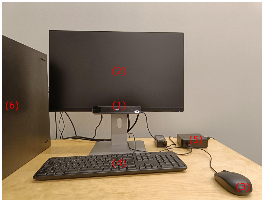
Figure 4.2 Picture of the eye tracker setup. Included in the picture is the eye tracker hardware, consisting of the camera and IR light (1), the monitor (2), mouse (3) and keyboard (4), as well as the eye tracker processing unit (5) and computer (6). Only gaze positions on the monitor were recorded.
