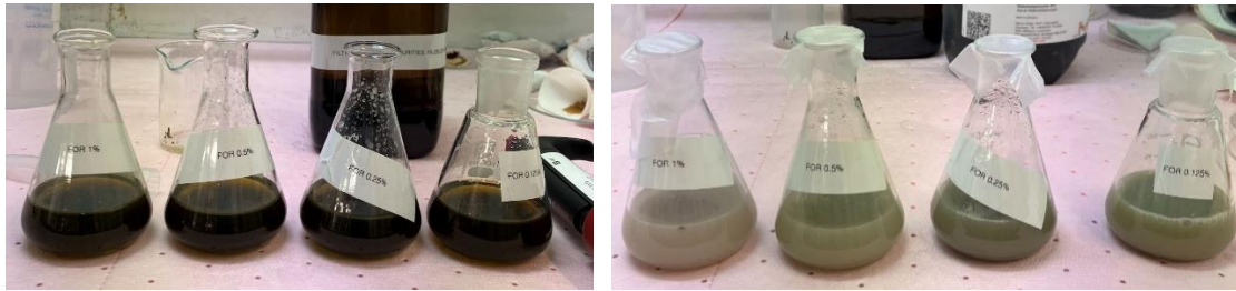
Figure 38. (a) Flasks with 50mL of PLS, (b) Flasks after adding and mixing the Hydrogen peroxide
