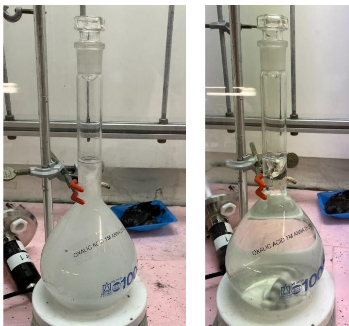
Figure 27. Dilution of Oxalic acid 1M, showing (a) recently started the dilution, (b) the end of dilution
