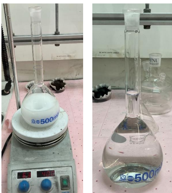
Figure 15. Dilution of Oxalic acid, showing (a) recently started the dilution, (b) the end of dilution
