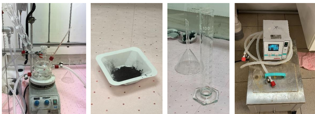
Figure 16. (a) Set up of the experiment, (b) Black mass weighed, (c) Graduated cylinder used to pour 100mL of Oxalic acid, (d) Heating circulator which I connected to the reactor
