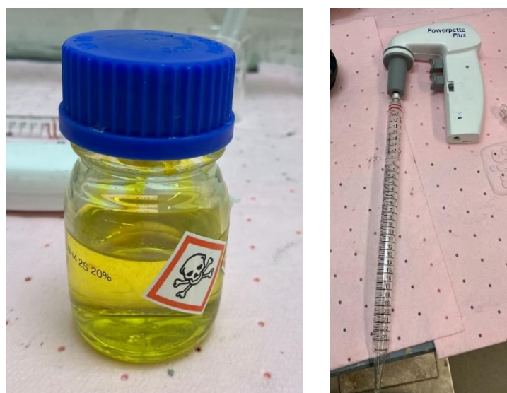
Figure 31. (a) Ammonium sulfide (\text{NH}_4)_2\text{S} , (b) Powerpette plus I used for adding the 50mL of the leachate to the reactor
