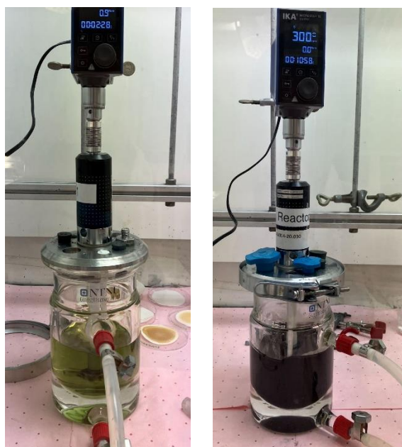
Figure 37. (a) Reactor before adding the ammonium sulfide, (b) Reactor after adding ammonium sulfide
