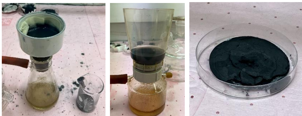
Figure 18. (a) Set up A of the filtering process, (b) set up B of the filtering process (c) precipitate obtained in the filtering process
