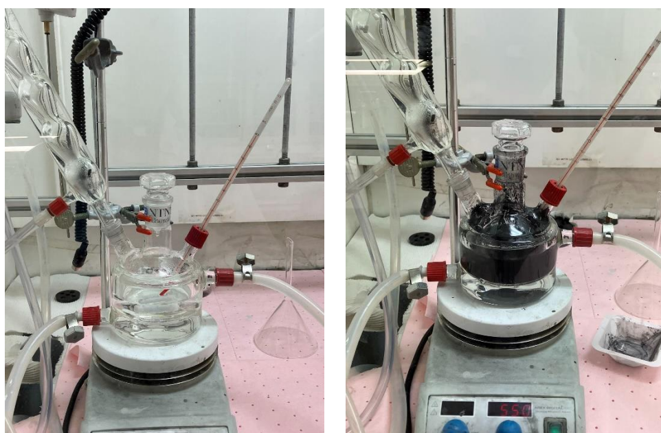
Figure 17. (a) Leaching process, showing (a) oxalic acid dilution heating to 80°C, (b) after pouring into the reactor the amount of black mass
