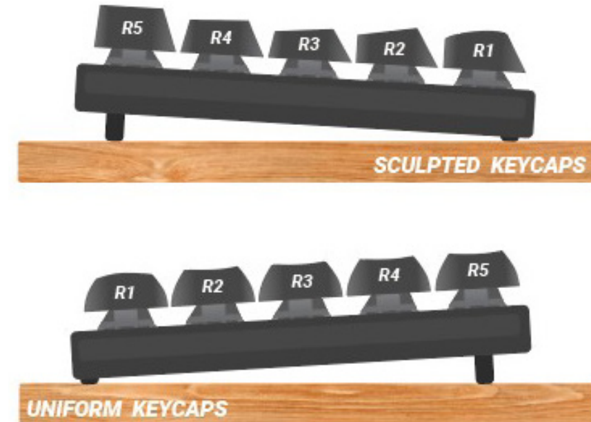
Figure 12. The differences between sculpted keycaps (top) and uniform keycaps (bottom) can be seen when compared side by side.
