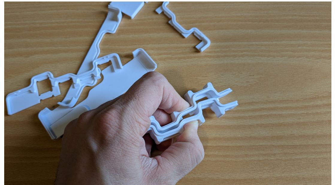
Figure 92. Prototyping the fit of the middle joint on the keyboard
