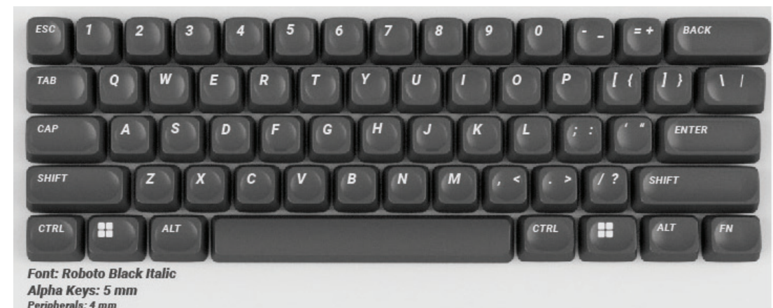
Figure 49. Final keycap design with final font
