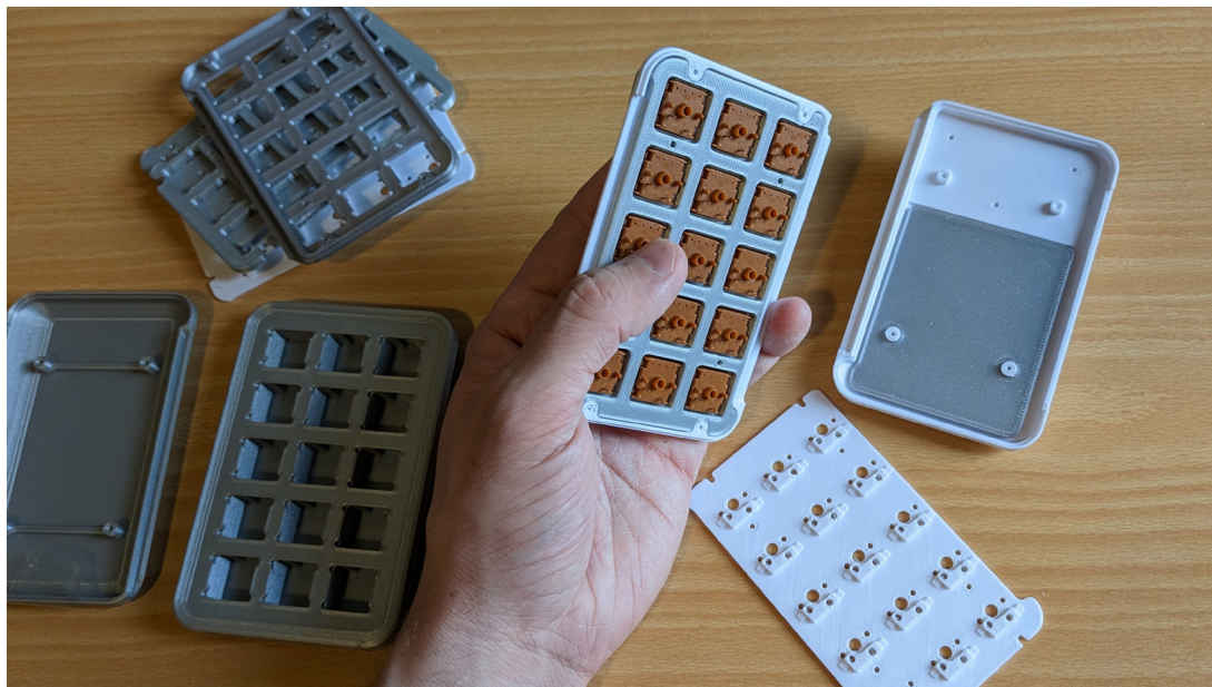
Figure 90. Prototyping all of the internal layers for the number pad.
