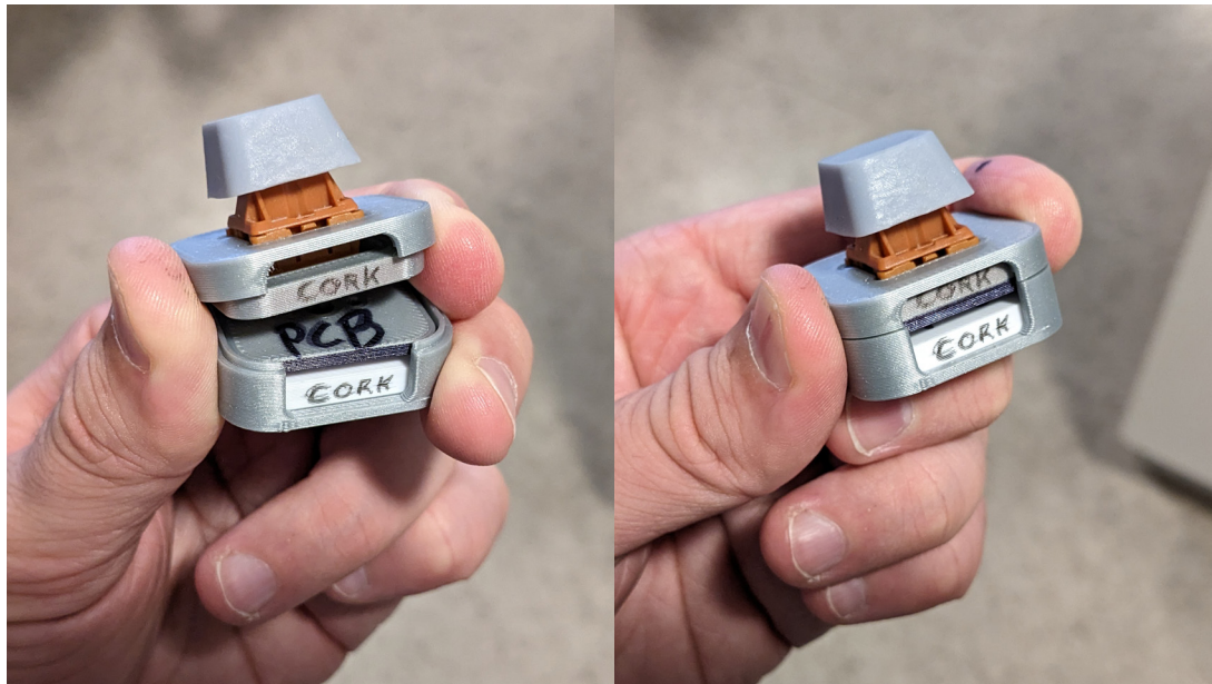
Figure 89. Prototyping keyboard internal layers.
