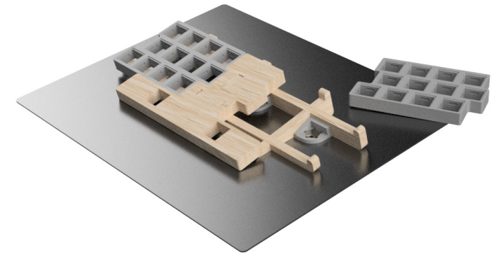
Figure 39. New keycap test rig allowed users to switch keycaps on the left side with the keycaps right side
