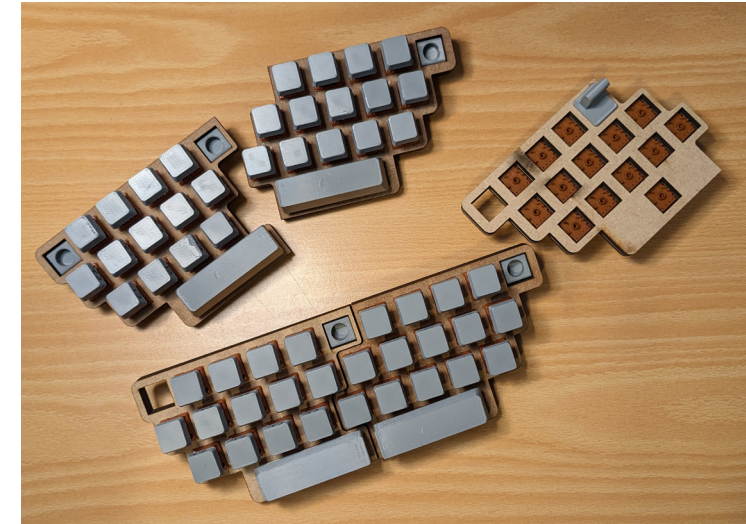
Figure 36. Test “half keyboards” were made to allow users to test different keycap angles side by side. Each half had a different keycap
