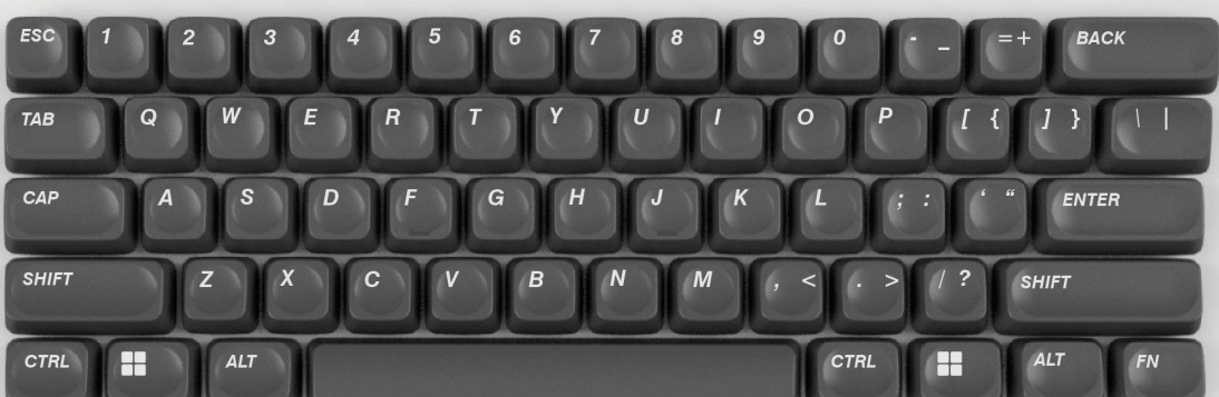
Font: Swis721 BT Alpha Keys: 5 mm Peripherals: 4 mm
