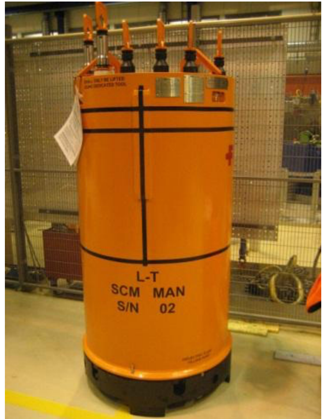
Figure 17. Picture of a subsea control module (Lervik, 2017)
