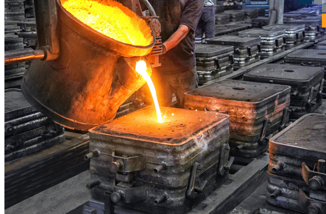
Figure 88. Picture of sand casting (Weld2cast, 2021)
