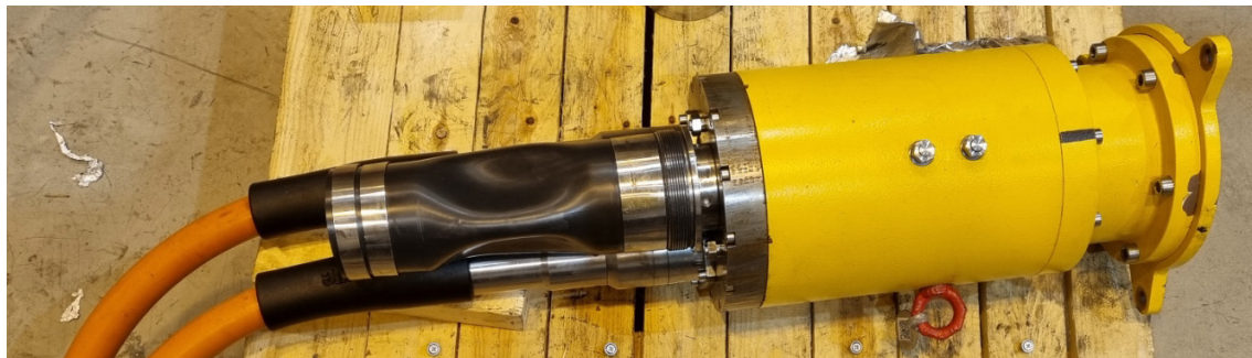
Figure 40. Picture of drive head (Private picture, 2023)
