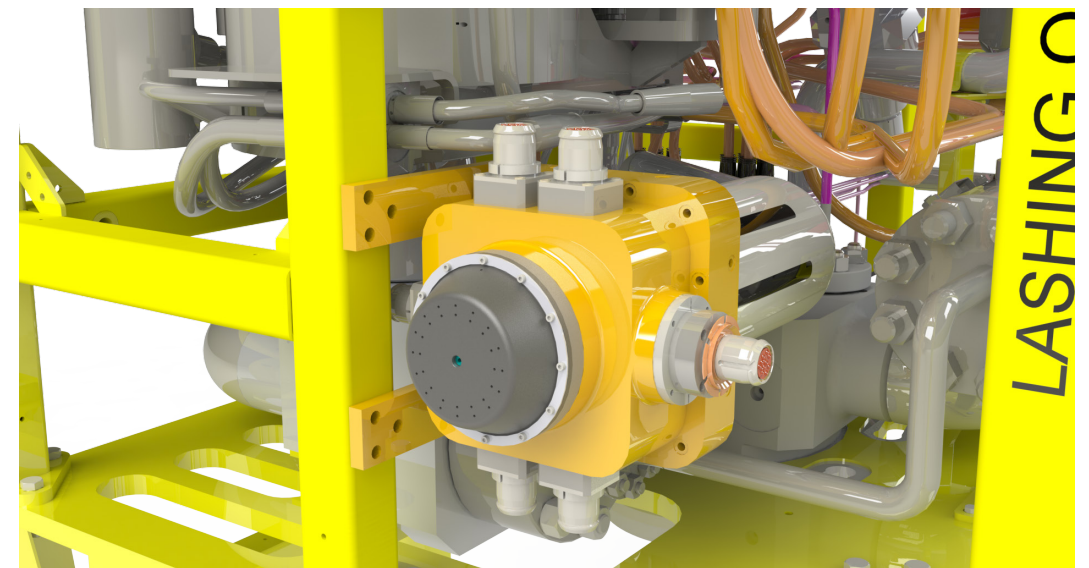
Figure 68. Horizontal fastening solution placed on FCM (Private picture, 2023)
