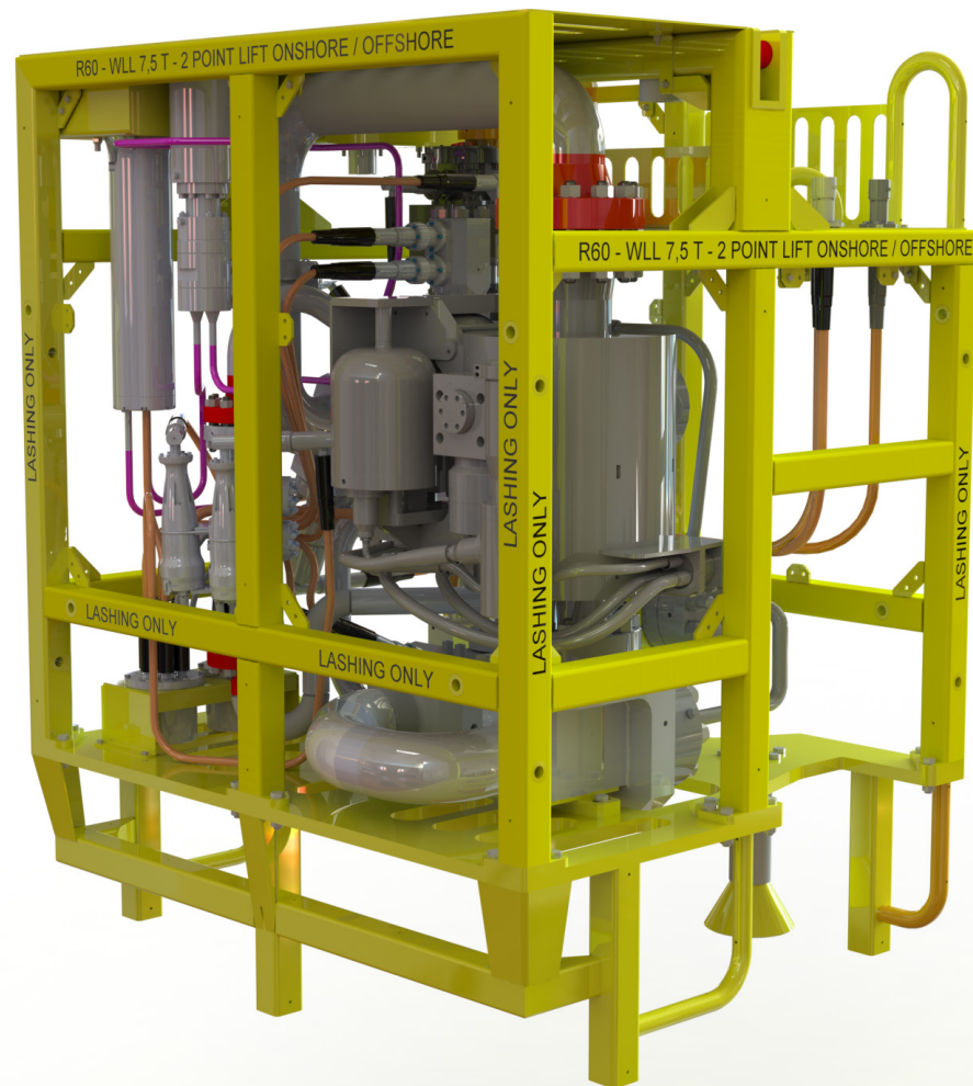
Figure 12. Render of hydraulic FCM (Private picture, 2023)
