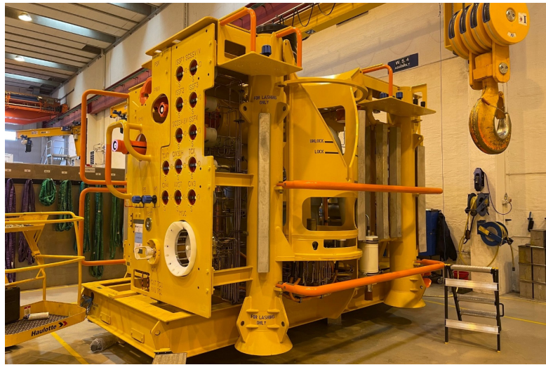
Figure 33. Xmas tree testing at Tranby (Dahl, 2021)
