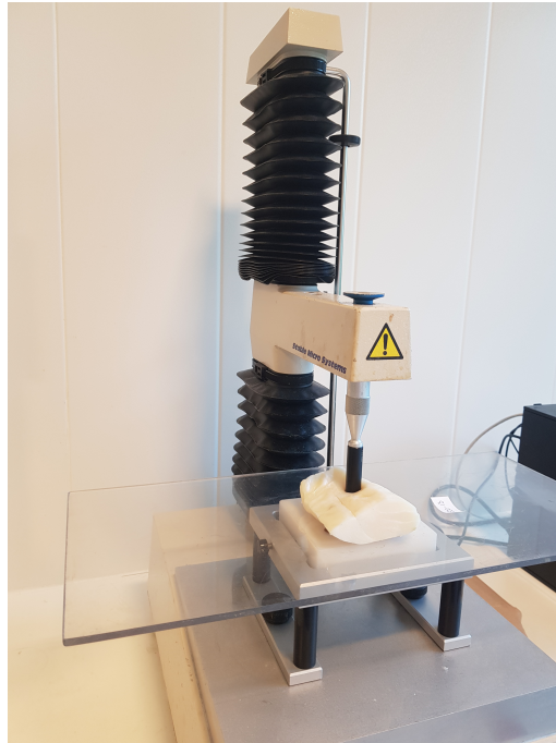
Figure 3.5: TA.XTplus texture analyzer setup.
