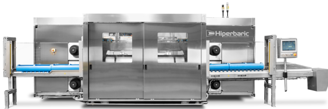
Figure 2.7: An illustration of an HPP system. The products are loaded into blue baskets which are then pushed into the vessel (holding chamber). Once inside, the vessel is sealed and water at a specific temperature is pumped in until the desired pressure is achieved. The pressure is maintained for a certain duration of time before it is released, allowing the product to emerge Credit: Hiperbaric ( Hiperbaric 55 n.d. )
