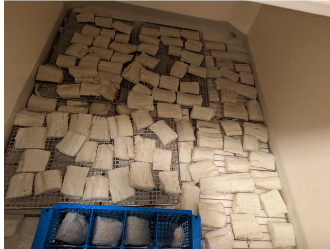
Figure 3.2: Clip-fish loins spread out in the polyethylene container. The loins in the blue basket were weighed and registered after 6, 12, 24, and 48 hours.
