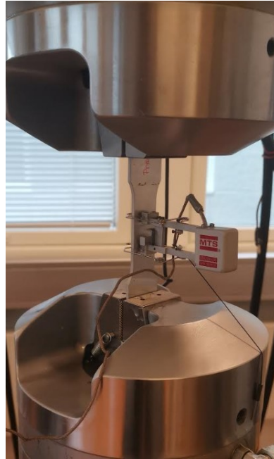
Figure 3.3: The setup for tensile testing with extensiometer for the rectangular sample.
