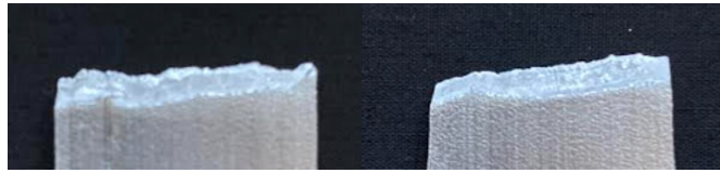
Figure 4.4: The fractures of Rectangular 1 (left) and Rectangular 2 (right).
