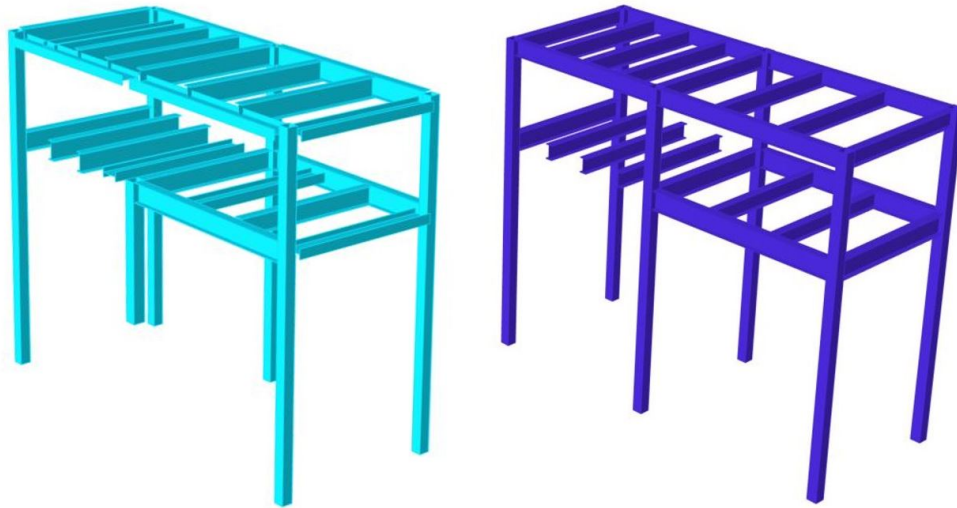
Figure 6.5: The figures represent the matched elements in the demand structure with substituted and original cross section, respectively.
