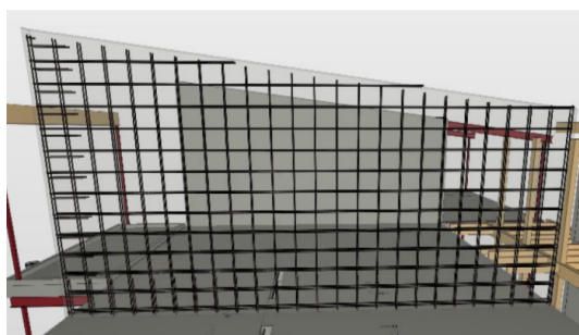
(a) Slakkarmering tilsvarende EC2 minimumskrav
