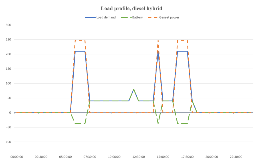
Figure 7: Load profile for Diesel Hybrid
