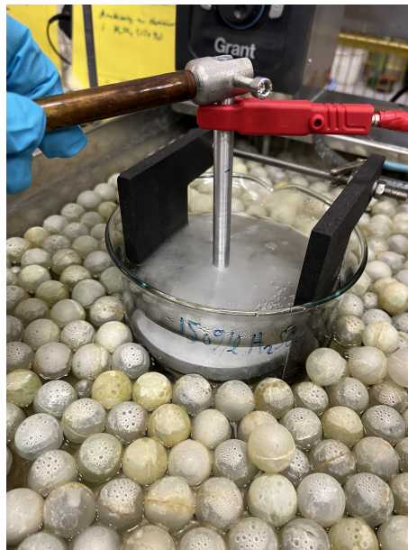
Figure 3.1: The anodising setup.
