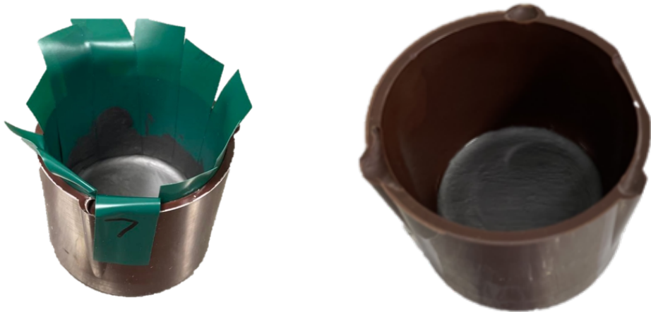
(a) Example of the conductive paint process. (b) Finalised manufactured insulation cup.
