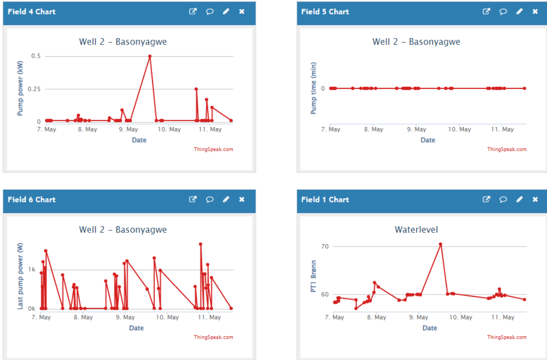
Figure 3.9: Plot from Thingspeak. The pump time and the pump power are not coherent, and the last pump power fluctuates a lot. The change in the water level still indicates that the pump has been on in accordance with the values in pump power.
