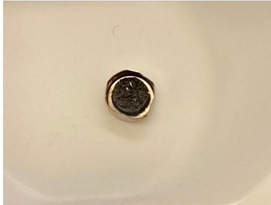
Figure 4-2: Photo of the sample with 1 molar ratio of \text{CaO}/\text{Al}_2\text{O}_3 after DSC.
