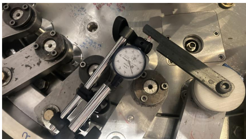
Figure 5.9: Dial gauge measurements on guide vane shaft.
