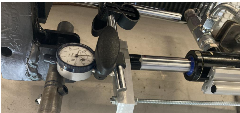
Figure 5.6: Dial gauge measurement on the backlash experienced in the second actuator joint.
