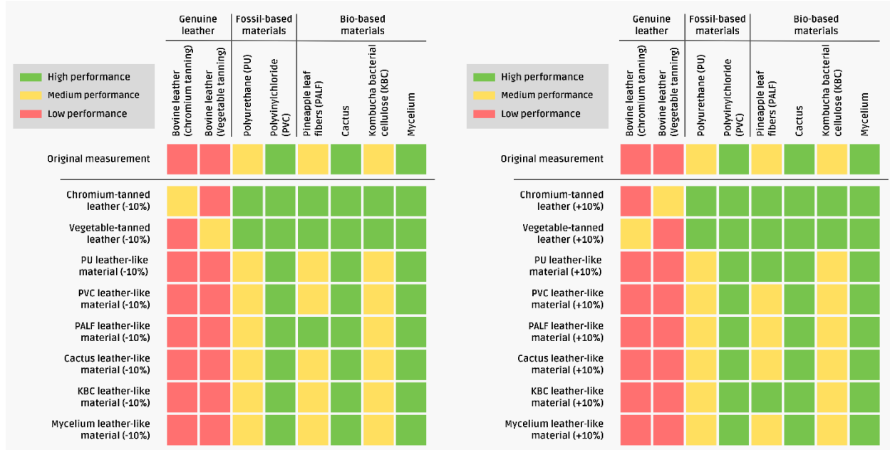
Figure S1 - Sensitivity analysis of the LiSET matrix for water consumption (in L/m 2 )
