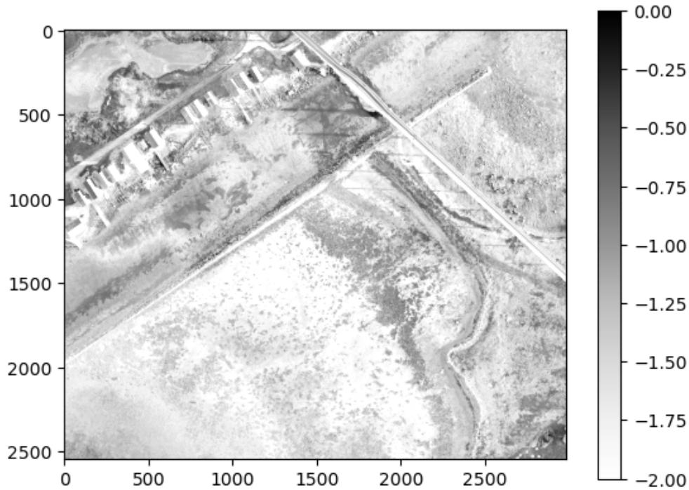
Figure 38: The spatial logarithmic error for the 32x32 SOM of the fused Remø. The SOM is trained for three iterations.
