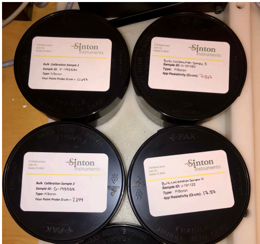
Figure 21: Bricks used for calibrating the BCT-300 instrument, in total 4 bricks. The known values of each brick can be found in Table 4.
