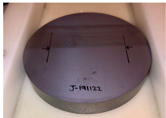
Figure 22: Brick used for brick calibration of BCT-300.
