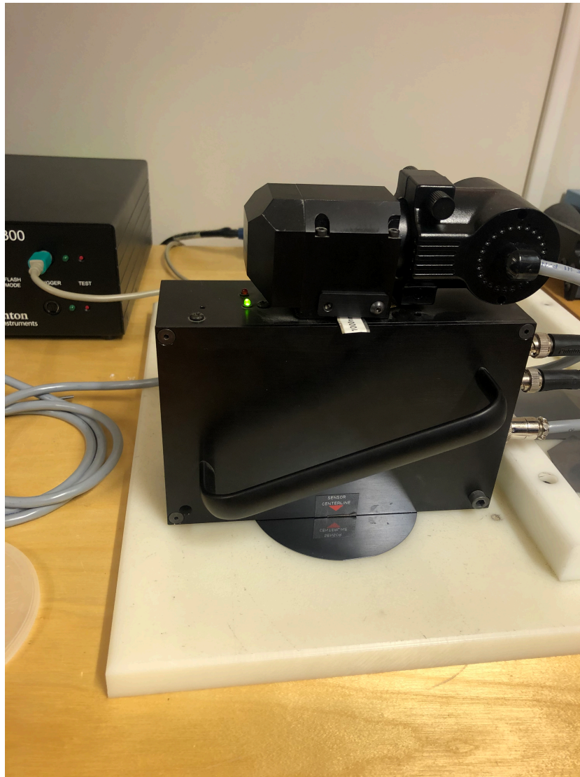
Figure 4.11: The figure displays the BCT-300, with the 1000 nm filter inserted, measuring a wafer. The BCT-300 shows a green LED light indicating that a stable internal Temperature has been reached.
