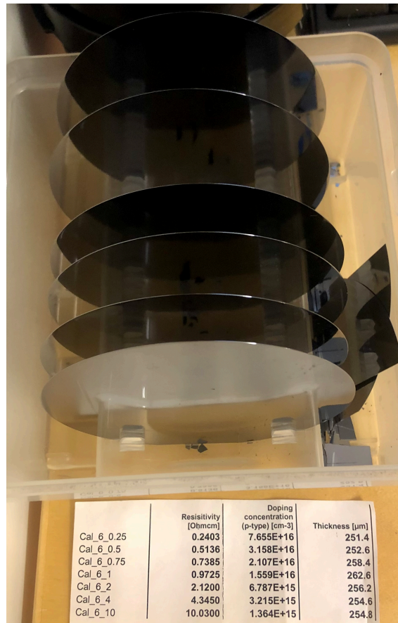
Figure 20: 6 wafers used for calibration of BCT-300, values can also be found in Table 4.
