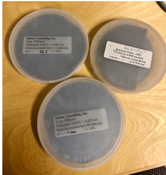
Figure 19: three reference wafers used to Qualify the tester.
