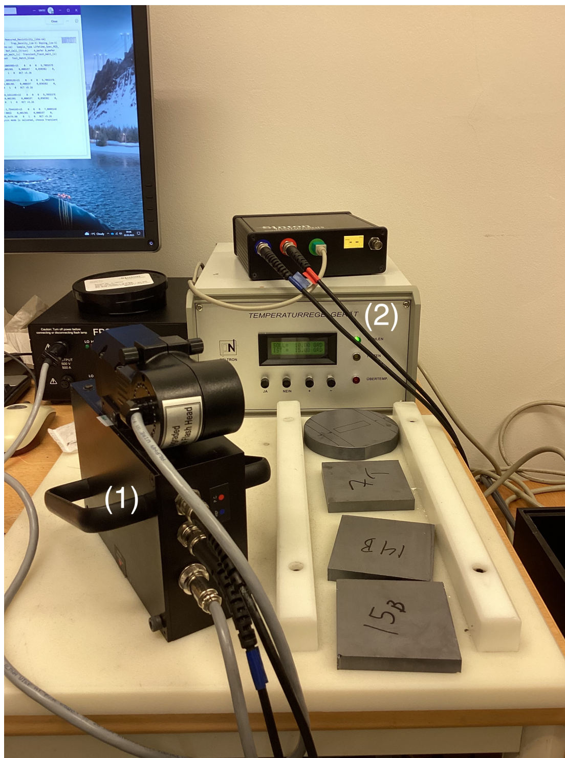
Figure 4.10: Part of the experimental setup which consists of the BCT-300 instrument (1) and temperature regulator (2).
