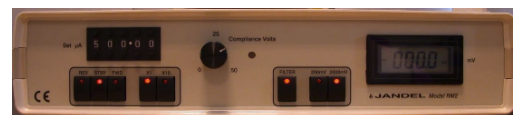
Figure 17: Steering Unit that allows changing the applied current and shows the output voltage measured on the sample.
