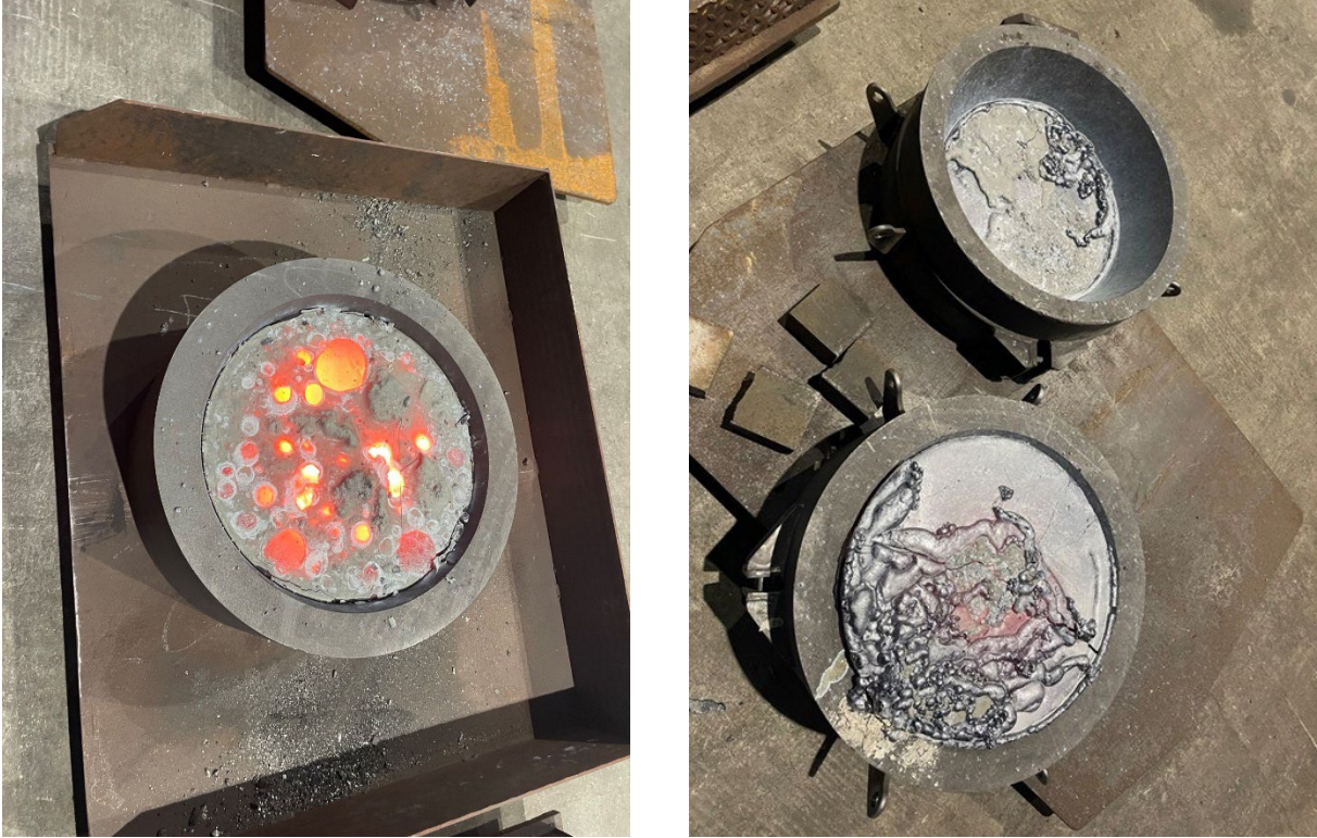
Figure 4.20: Left: Slag tapping where metal pearls are visible on the top of casting as round pearls. Right: Solidified metal tapping.
