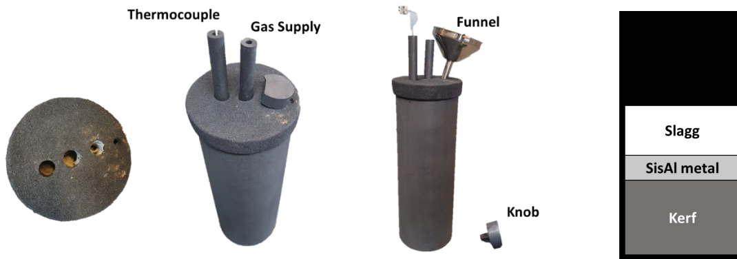
Figure 3.4: To the left: Picture of the lid used in the experiments. In the middle: picture of the setup in the crucible, with lid, graphite tube to protect the thermocouple, and gas lance. The last hole is covered with a knob during heating, and a funnel is inserted when quartz is added. To the right: the stacking of raw materials in the furnace.
