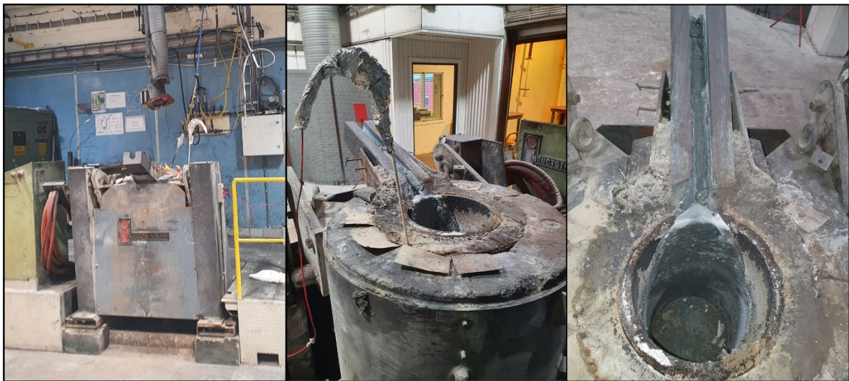
Figure 3.7: Pictures of the furnace used for the medium-scale trials. The furnace was a 225-kW induction furnace, with a 40 liters crucible, and a tap chute. To the right, the leftovers from an experiment can be seen in the crucible and chute.
