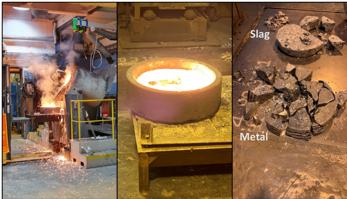
Figure 3.8: To the left: Casting of material. The furnace is tilted, and the mold is elevated. In the middle: The hot metal is left in the molds to cool down. To the right: The metal was cast in the first mold and the slag in the second. The products were removed from the molds and left on the floor for the remainder of the cooling period.
