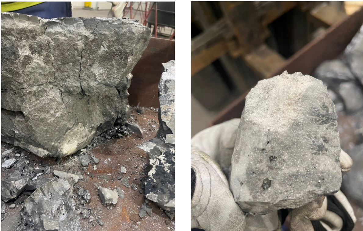
Figure 4.19: Undissolved lumps visible in the slag tapping.
