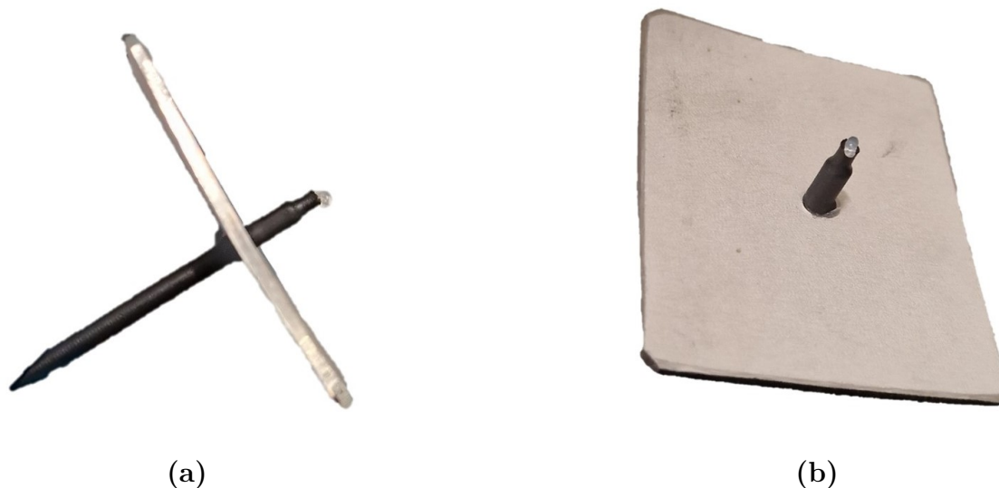
Figure 4.7.: Specimen mounting on threaded rods. Heat shrink tubing and silicone were used to shield the threaded rod, and the connection between the sample and rod.
