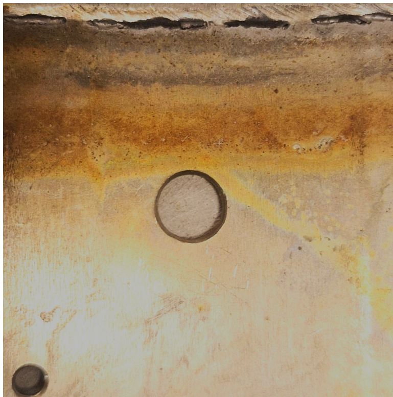
Figure 4.9.: One of the samples scanned by SEM and analyzed by EDS. This is the sample exposed to the potentiostatic test at 400mV 2°C.
