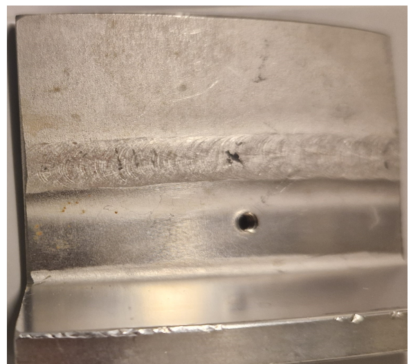
(f) Good Weld.
