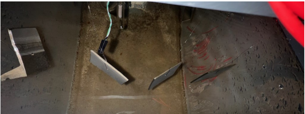
(b) Free surface AISI 316L samples.
