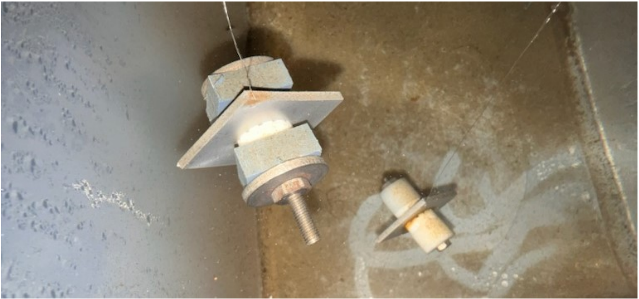
(a) Corrosion on crevice samples.
