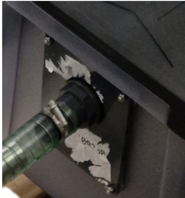
Figure 3.3.: Support for the inlet valve assembly, constructed and implemented for the setup at InnovaNor.
