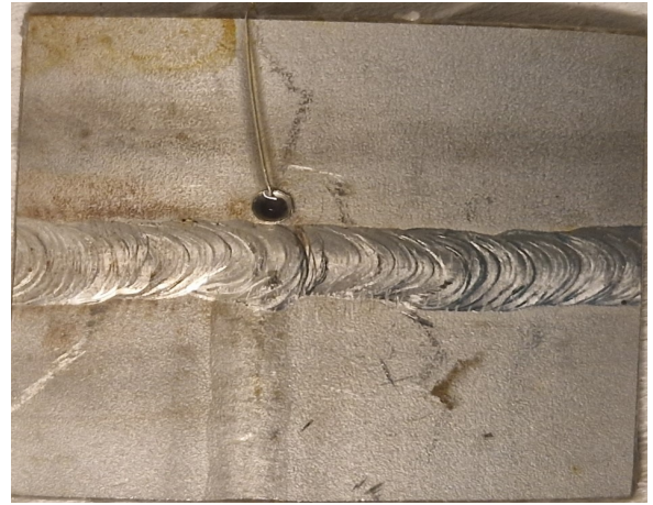
(b) Bad Weld Outside.
