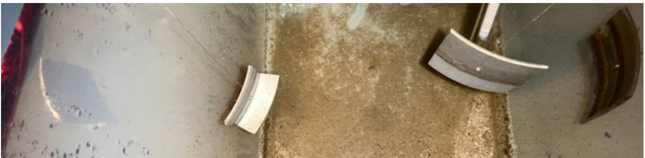
(c) Welded samples without visible corrosion.
