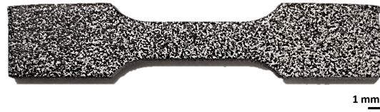
Figure 4.1.2: Dogbone specimen after cutting and painting.
