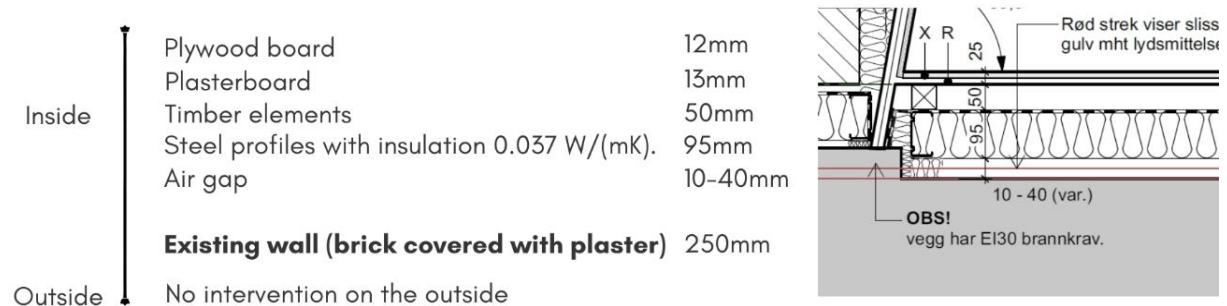
Figure 15 Technical detail external wall of the intervention at Voldsløkka school (Taken from ARK documents from Voldsløkka school project)
