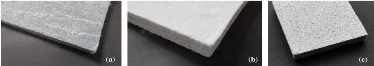
Figure 19 Available aerogel (a) Spaceloft blanket, (b) Heck AERO board, (c) Fixit 222 render (Taken from Aerogel materials for heritage buildings: Materials, properties, and case studies)
