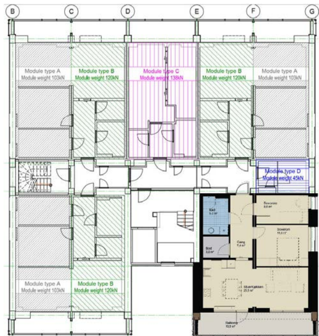
Figure 9 Kodumaja's prefabricated modules and plan, image source: (Malo et al., 2016), own drawing in Revit
