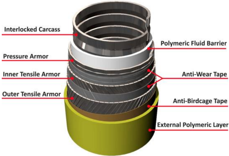
Figure 0.1. The cross-section of an unbonded flexible pipe [3].
