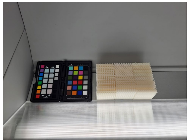
Fig. 17 Appearance and accuracy of gradient lattice-based structures in as-printed SLA samples using PrimaCreator Value resin. After 12 h, a yellowish color began to appear
