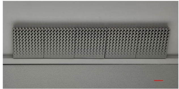
Fig. 7 Appearance and accuracy of gradient lattice-based structures in as-printed FFF samples using PLA filament and Prusa i3 mk3s+ (scale bar represents 1 cm)
