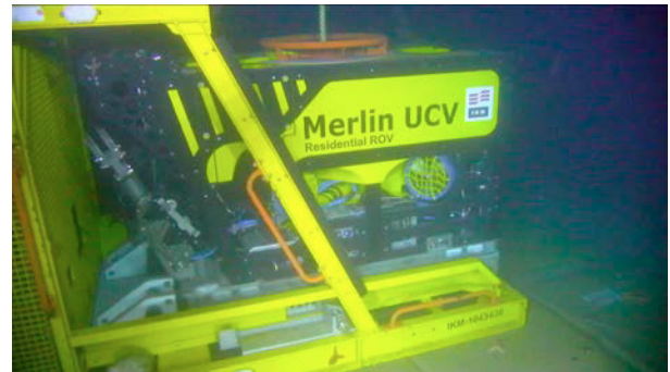
Fig. 2. A Merlin Resident ROV with its “garage” from IKM. Image courtesy of IKM.
