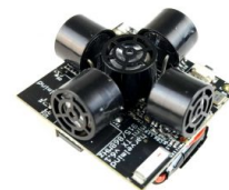
(b) Marvelmind Mini TX without its casing
