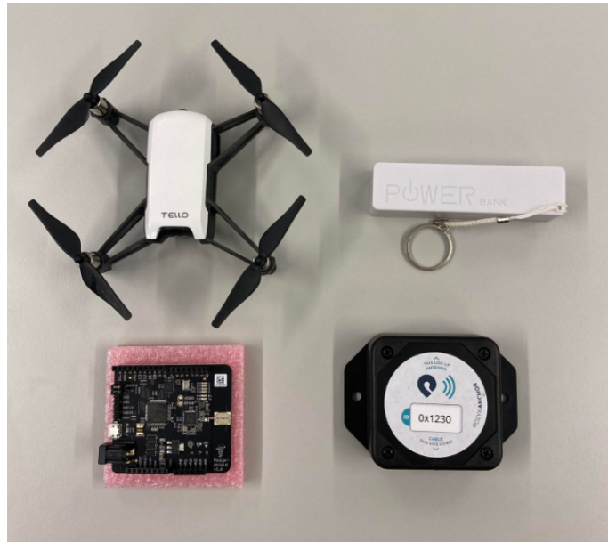
Figure 3: Creator One kit + Tello Drone, top left is Tello drone, Battery pack, mobile beacon, and anchor.
