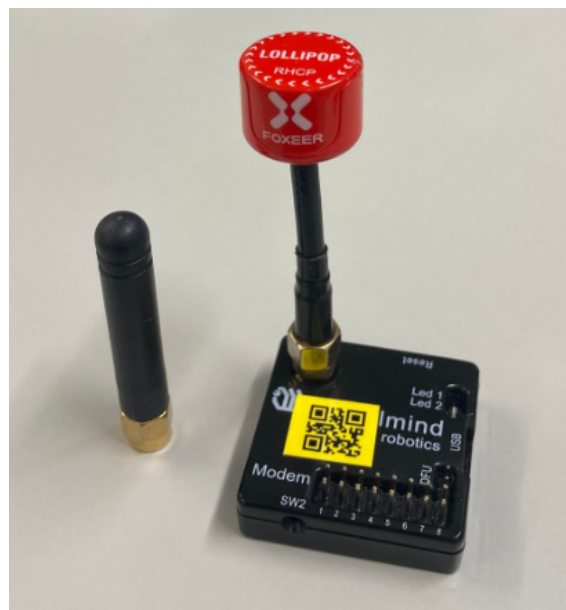
Figure 56: Different antennas on the Marvelmind modem [11]
