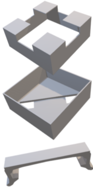
Figure 16: Computer model of the container to the Marvelmind node mounting to the drone.
