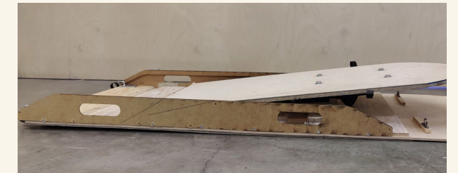
Figure 72. Gas spring installed in the mockup stretcher. Testing minimum angle.
