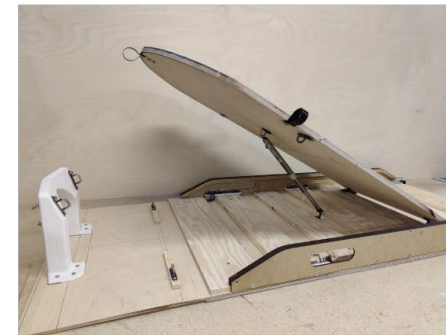
Figure 39. Prototype of the gas spring.
