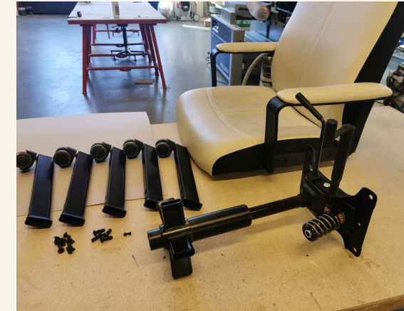
Figure 70. Using an old office chair to find a blockable gas spring.
