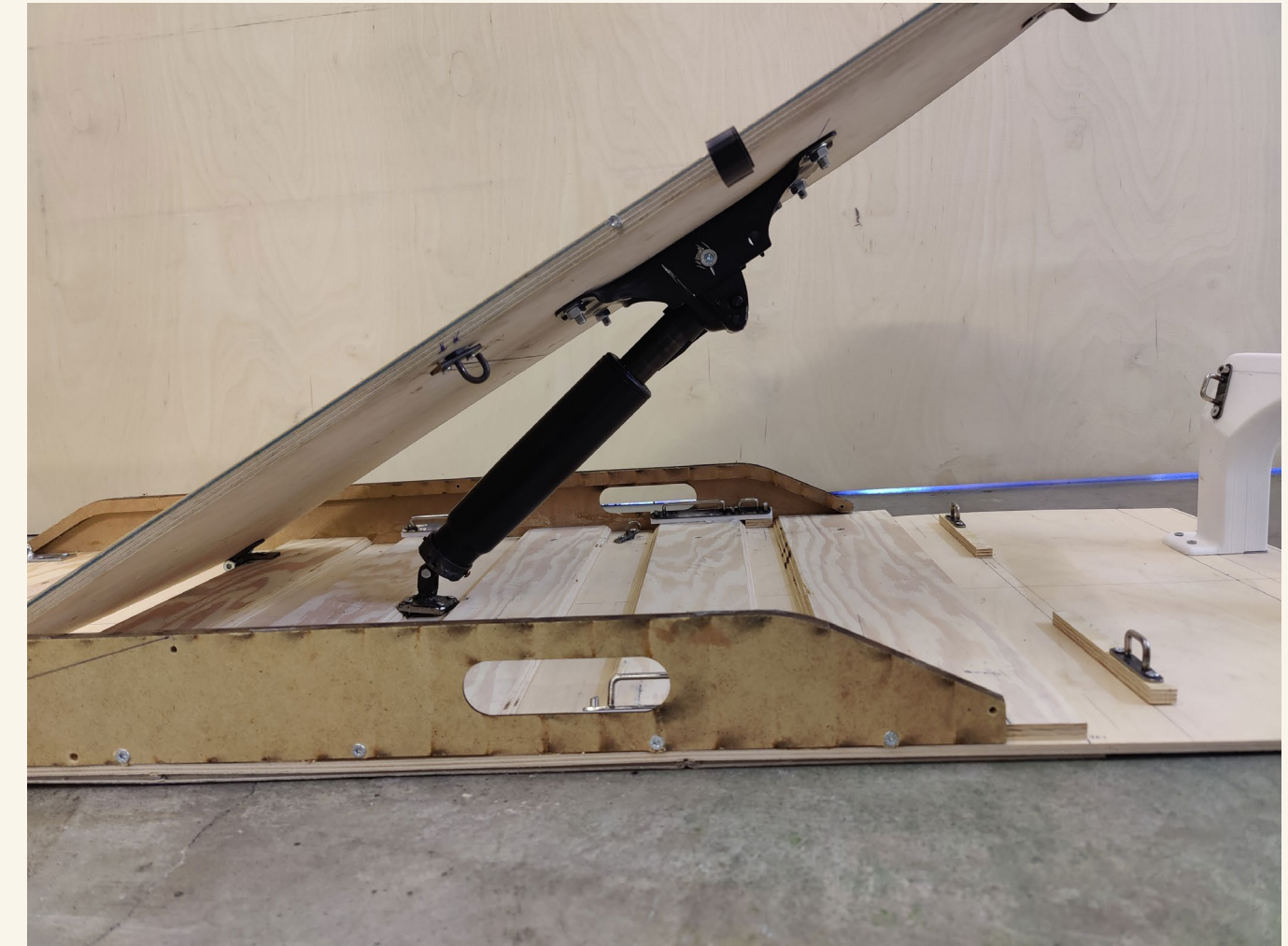
Figure 73. The final concept for the elevation mechanism.
