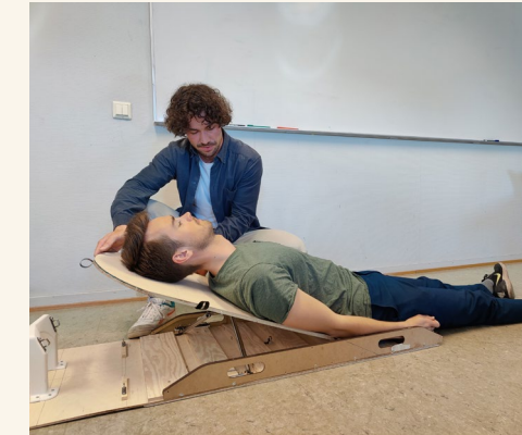
Figure 56. This was the preferred position when focusing on ease of lifting while maintaining good overview and access to the patient while not being in the helicopter.
