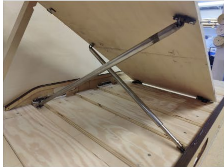
Figure 43-45. Prototype of the diagonal gas springs in the mockup.
