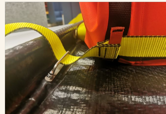
Figure 15. Closeup of how the rescuebag strap is fastened to the bracket.
