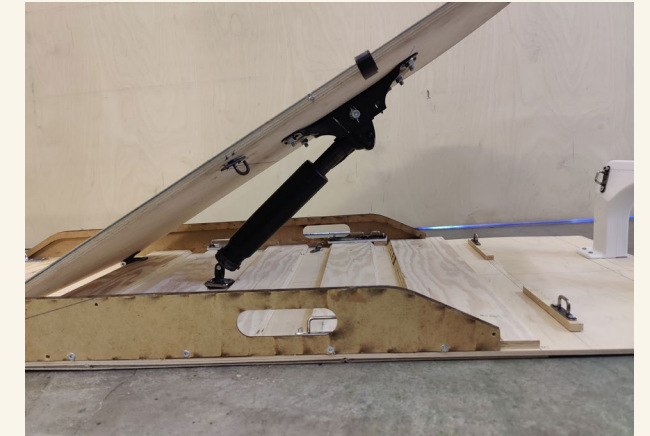
Figure 71. Gas spring installed in the mockup stretcher. Testing maximum angle.
