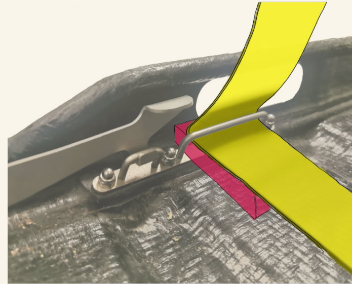
Figure 102. Illustration of fastening mechanism beneath the strap. Creates a risk of jamming the strap.
