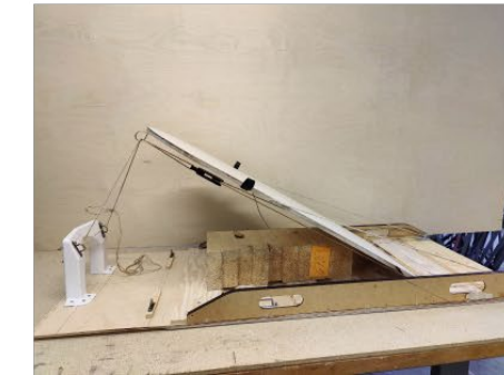
Prototype with rope and a 3D-printed pulley.
