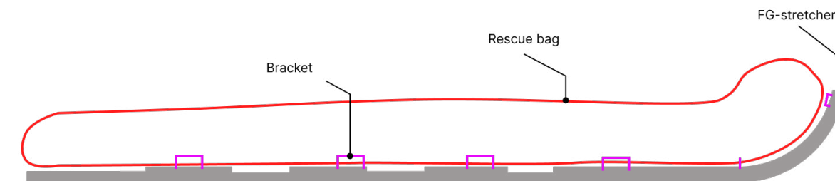
Figure 88. Section view - side. FG-stretcher and rescue bag
