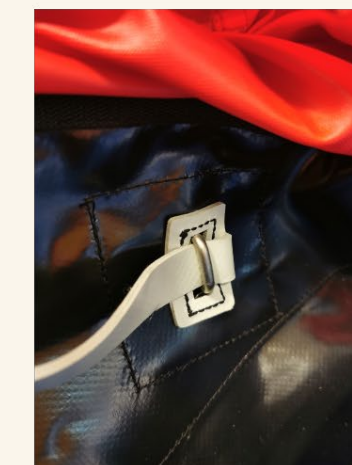
Figure 16. Closeup of how the head part of the rescuebag is fastened to the bracket.
