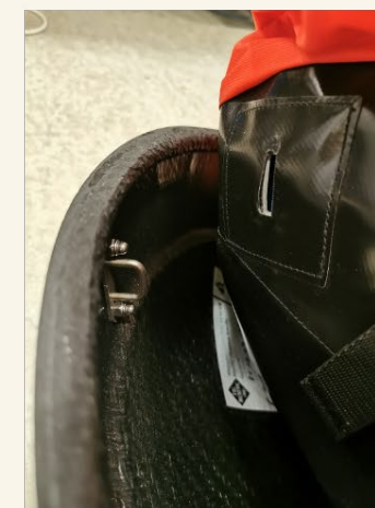
Figure 16. Closeup of how the head part of the rescuebag is fastened to the bracket.
