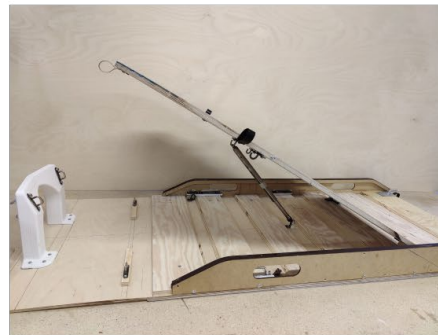
Figure 40-41. Prototype of the gas spring in the mockup.
