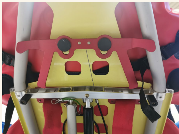
Figure 117-118. Operating handle of the AC-stretcher.
