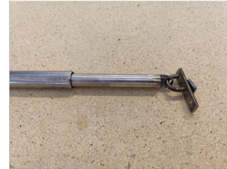
Figure 39. Prototype of the gas spring.
