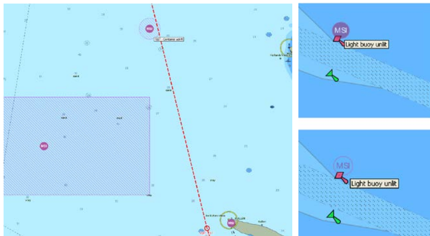
Figure 2. Example of portrayal of MSI integrated in the ECDIS display. Left, two Area MSIs and a point MSI, right, an unacknowledged MSI (top) and an acknowledged MSI (bottom).
