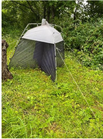
Figure 2: The setup of the malaise traps (SLAM, standard type II) that was used to collect the arthropod data in this study. The sloped white roof guided the arthropods to the container at the top of the trap with 96% ethanol. Photo: Margrete Saugestad (Sleneset, 2022).
